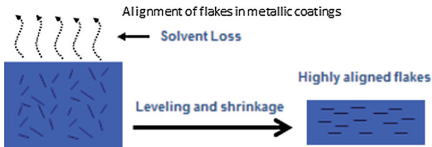
Fig. 13.6 Flakes in metallic basecoats align preferentially with the surface of the coating due to shrinkage in the thickness direction as solvent evaporates from the coating surface. Improved flake alignment leads to improved metallic appearance
