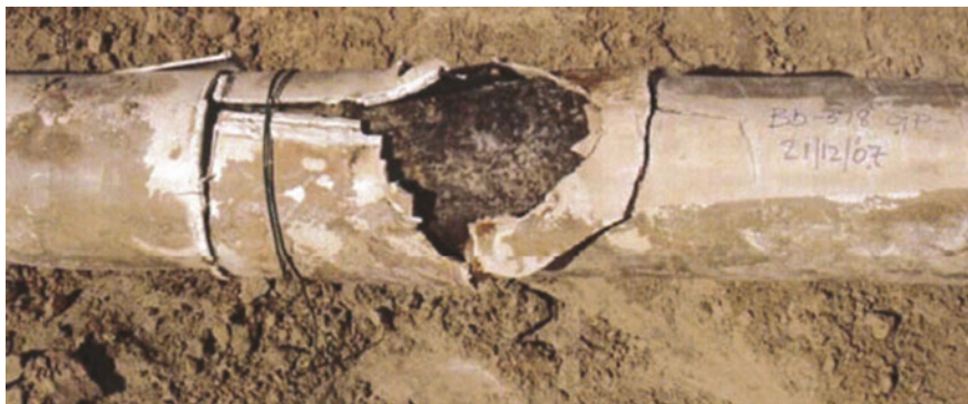
Fig. 14.18 Crack and disbonded field joint polypropylene [76]
