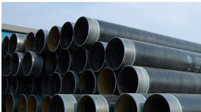
Fig. 14.1 3 layered polyethylene (3LPE) coated pipes; note the ends of the pipes are exposed to facilitate joining by welding
