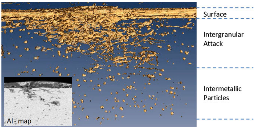
Fig. 10.6 Reconstruction from Al elemental maps of an attack site in AA2024-T3 beneath filiform corrosion (A. M. Glenn and A.E. Hughes, unpublished)
