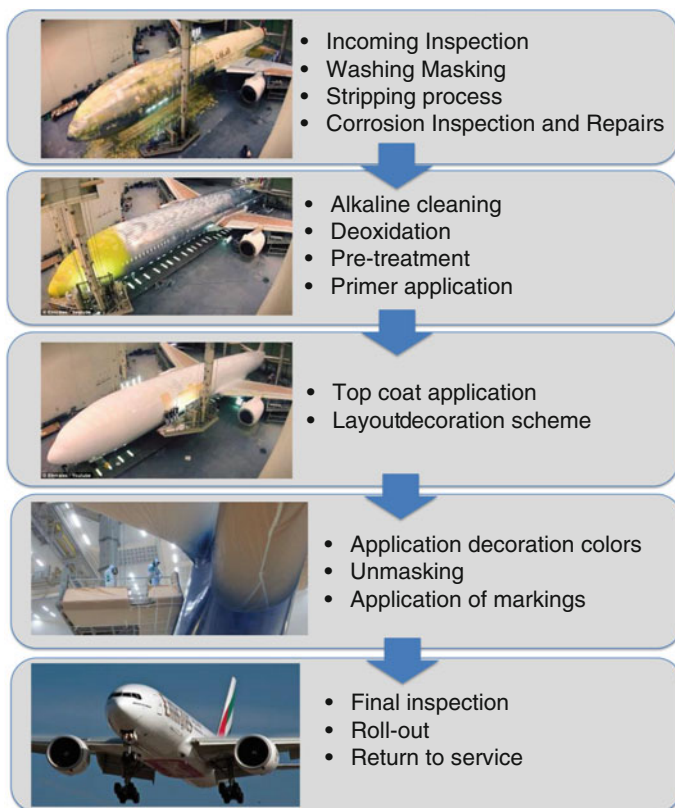
Fig. 12.11 Steps required for aircraft painting (images kindly provided by Airbus and Emirates Airlines)
