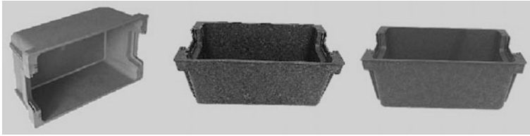
Fig. 8 Comparison of colouring of different fiber types (wood left ; flax middle ; hemp right )
