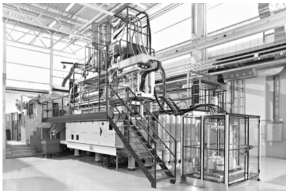
Fig. 7 Injection molding compounder at Fraunhofer Pilot Plant Center Schkopau (Michel 2015)
