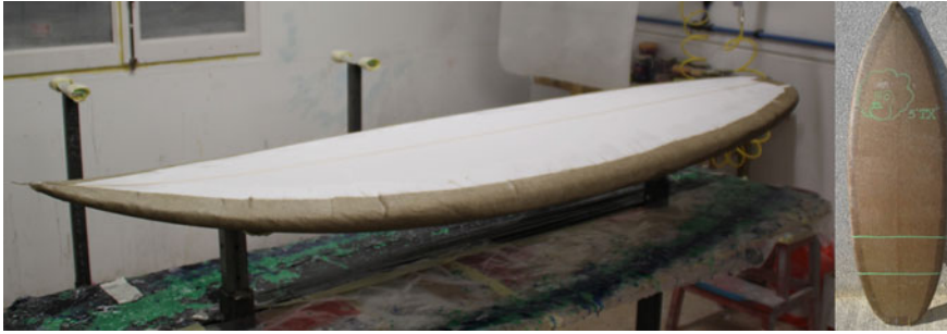
Fig. 9 Surfboard prepared for deck lamination ( left ) and finished ( right )
