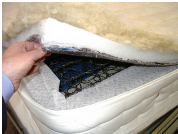
Fig. 5 Mattress insulator pad (grey layer) produced from a blend of recycled wool and mixed fibres to protect against spring penetration
