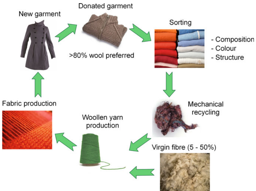
Fig. 6 Example of closed loop mechanical recycling of wool garments
