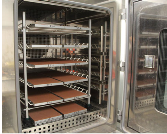
Fig. 4 Climatic chamber with mortar samples for adsorption and desorption test
