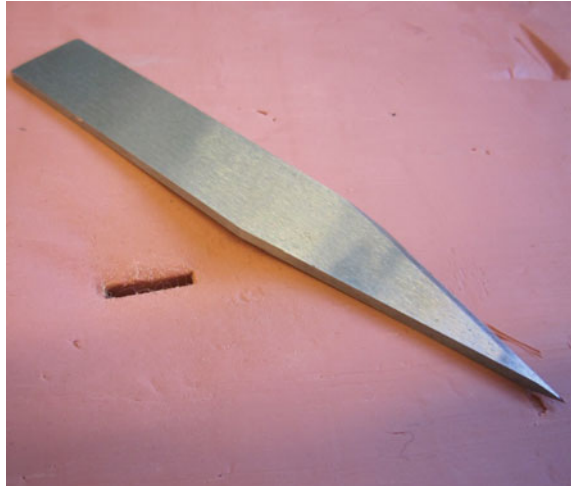
Fig. 2 Knife of specific dimensions and sharpness for stab resistance (from Weber et al. 2014a)
