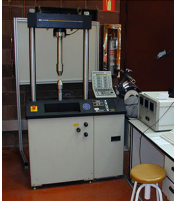
Fig. 2 Universal test machine Instron 8516 used to carry out the tensile tests
