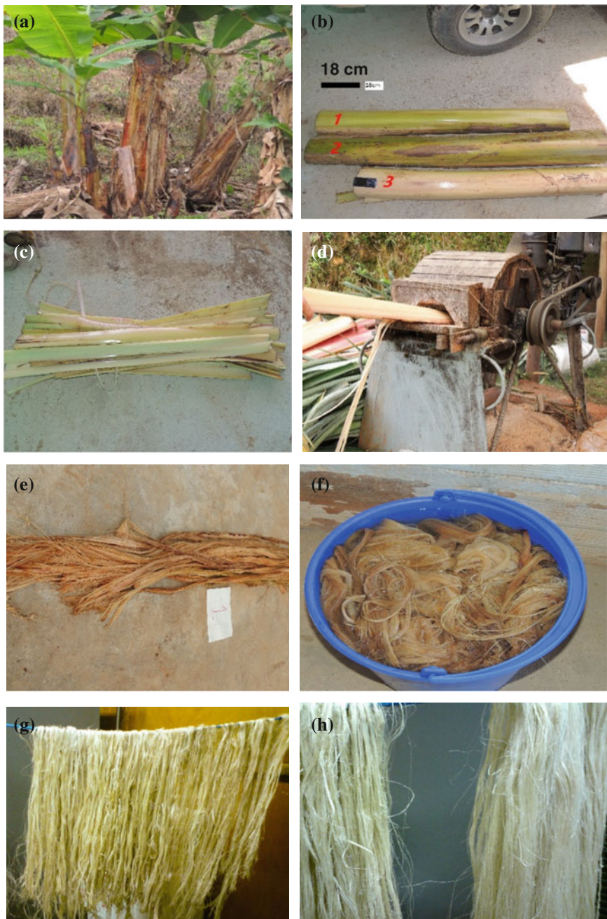
Fig. 4 Mechanical extraction process of the plantain fibers. a Pseudostem after harvesting the fruit. b Collected pseudostems. c Unsheathing. d Extraction of fiber. e Wet fiber extracted. f Fermentation process. g Drying. h Combing of the fibers
