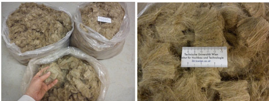
Fig. 1 Primary bast hemp ( Cannabis Sativa L.) fibres cut in form of fibre reinforcement for concrete
