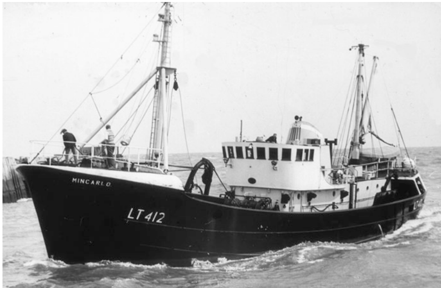
Fig. 4 Lowestoft trawler Mincarolo , built in 1960–1961 and characteristic of side-winding diesel trawlers built during the 1950s–1960s. Currently a museum vessel stationed in Lowestoft harbour (Photo: Crown Copyright)
