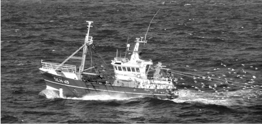
Fig. 5 Dutch trawler in action, characteristic of mechanised twin-beam trawlers (Photo: Georg Engelhard)
