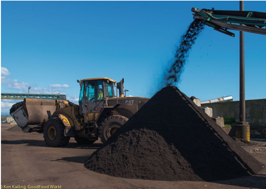
Fig. 4 Screening the finished compost product. Screening to different particle sizes allows us to develop products for different markets. It also assures the consistency of the product
