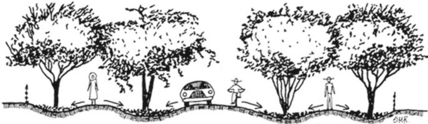
Fig. 7 Raise pathways, and sink mulched and vegetated basins (Illustration by Ann Audrey and reproduced with permission from Rainwater Harvesting for Drylands and Beyond , Volume 1, 2nd Edition, by Brad Lancaster)
