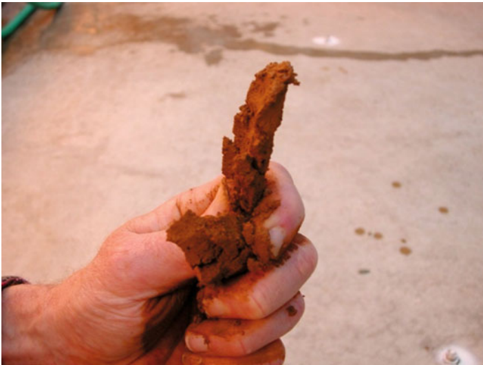
Fig. 6 Estimating soil texture by hand. The long soil ribbon shows that this sample is rich in clay (Photo by Andy Bary)
