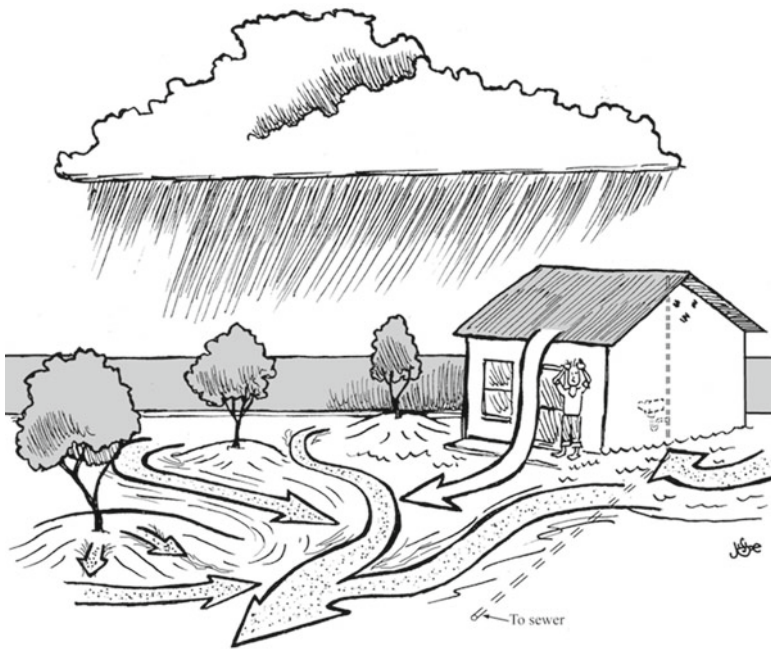
Fig. 1 The wasteful path to scarcity. The site rapidly dehydrates itself by erosively draining rain-water and runoff to flood downslope areas and contaminate surface water with sediment. Greywater is lost to the sewer. Costly municipal or well water is pumped in to replace the free water that was drained away. Leaf drop/mulch is also raked/drained away, further reducing fertility and water-holding capacity. This leads to a depletion of resources and feeling “scared in the city” due to the resulting scarcity (Illustration by Joe Marshall and reproduced with permission from Rainwater Harvesting for Drylands and Beyond, Volume 2, by Brad Lancaster)
