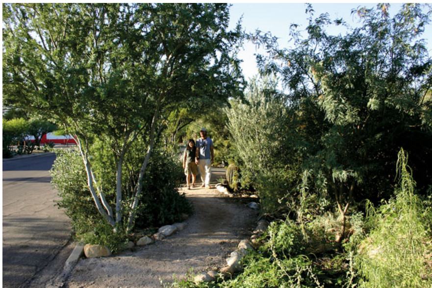
Fig. 4 After planting of rain and trees. Tree-lined footpath reviving the once-sterile right-of-way, 2006. Plants are irrigated solely with passively harvested rainwater and street runoff in Tucson, Arizona, where annual rainfall averages 11 in. (Reproduced with permission from Rainwater Harvesting for Drylands and Beyond , Volume 1, 2nd Edition, by Brad Lancaster)
