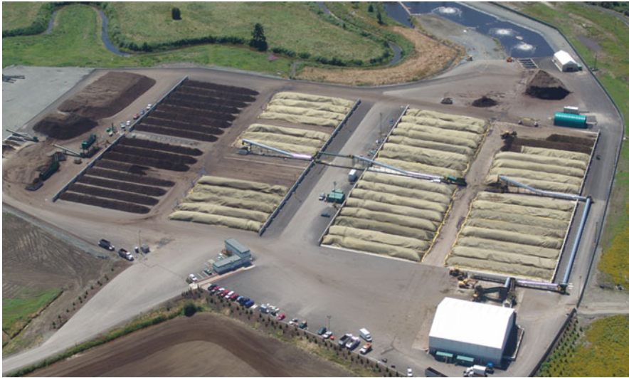
Fig. 2 An aerial view of the Cedar Grove composting facility in Everett, WA. The Gore covers are visible on the actively composting windrows. The curing piles are open to the atmosphere. The feedstock receiving building is shown on the bottom right of the photo
