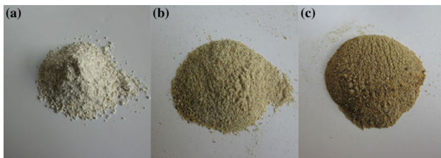
Fig. 6.12 Appearance of Fuzi before and after steam explosion. a Raw Fuzi. b 0.6 MPa. c 1.0 MPa
