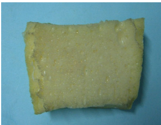
Fig. 6.29 Polyurethane foam produced by liquefied product of steam-exploded straw
