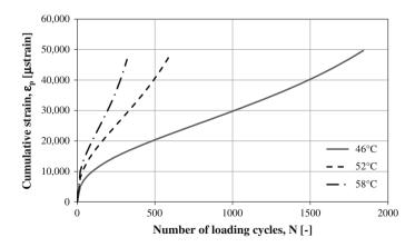
Fig. 5 Results of FN tests carried out on mixture M-B1 at all test temperatures
