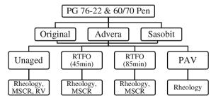
Fig. 2 Experimental matrix for modified and unmodified binder mixed with WMA additives
