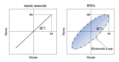
Fig. 4 Loading cycle in a strain-stress diagram for a perfectly elastic material (*left*), and for a viscoelastic material, such as hot mix asphalt (HMA) (*right*)
