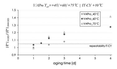
Fig. 4 Change in dynamic modulus |E\*| of lab-aged HMA specimen relative to unaged condition
