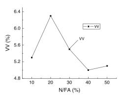
Fig. 2 N/FA versus the total voids in mineral aggregate (VMA)
