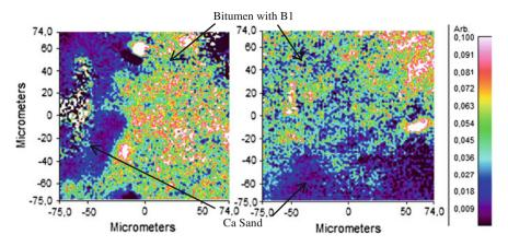
Fig. 4 FTIR-ATR microscope  $1030 \text{ cm}^{-1}/(1460 + 1376 \text{ cm}^{-1})$  band ratio images for mastic aged for 14 days in oven 7.5 % B1 added
