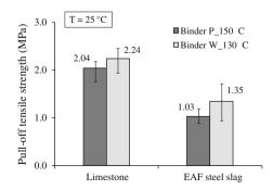
Fig. 3 BBS mean test results
