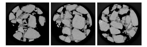
Fig. 5 Example of CT-scans of LEAB-PA16+ after laying (3 different heights of the core)
