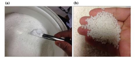
Fig. 1 a Advera $\mbox{\ensuremath{\mathbb{R}}}$  WMA additive acquired from PQ Corporation. b Sasobit $\mbox{\ensuremath{\mathbb{R}}}$  WMA additive acquired from Sasol Company
