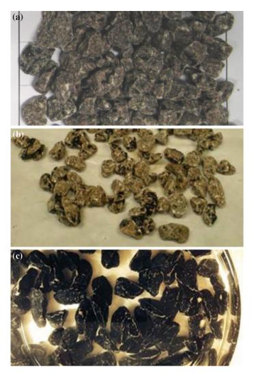
**Fig. 3 a.** Pictures of granite aggregate with PmB after 24 h from lab 1 with 5 % coating. **b.** Pictures of granite aggregate with PmB after 24 h from lab 4 with 20 % coating. **c.** Pictures of granite aggregate with PmB after 24 h from lab 3 with 40 % coating
