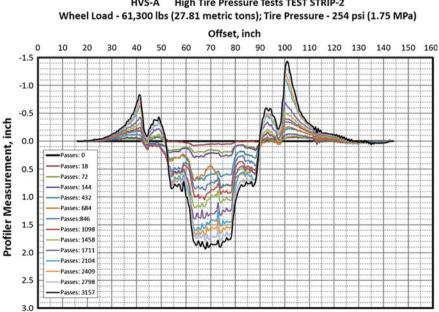
High Tire Pressure Tests TEST STRIP-2 HVS-A
