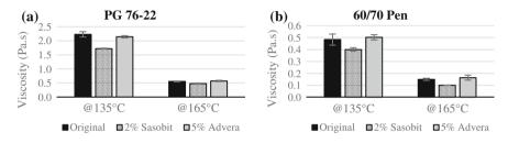
Fig. 8 Viscosity measurements for a PG 76-22 b 60/70 Pen asphalt binders mixed with WMA additives
