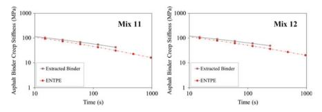
Fig. 5 Back-calculated and extracted creep stiffness of asphalt binder: mix 11 and 12
