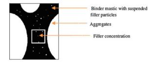
Fig. 1 A 2-D conceptualization of filler concentration
