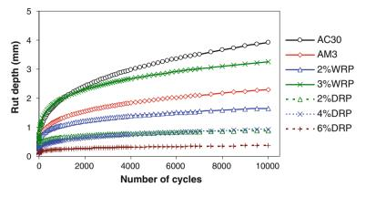
Fig. 5 Evolution of the rut depth for the analyzed mixtures
