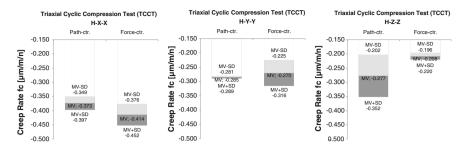
Fig. 8 TCCT results-path- versus forced-controlled compaction: creep rates
