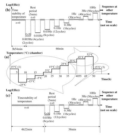
Fig. 2 Temperature chronology of each test (a) and chronology of frequencies at each temperature: 35, 45 and 52 °C (b) and from 10 to 25 °C (c). All cyclic loadings at fixed strain amplitude of 50  $\mu$ m/m
