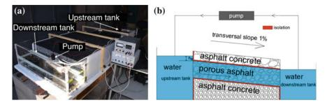
Fig. 3 Laboratory mock-up photograph (a) and operating schema (b)
