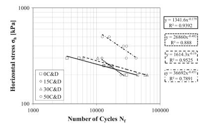
Fig. 4 Fatigue curves in terms of horizontal stress as a function of number of cycles
