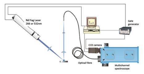
Fig. 5 Instruments used in a LIBS system
