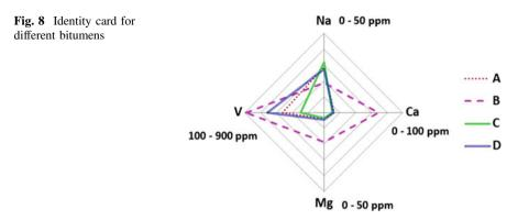
between certain bitumens in a clear and statistically significant manner, as well as to establish with certainty when there is any variation in the metal content of our bitumens.
