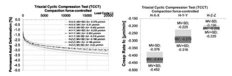
Fig. 6 TCCT results for force-controlled compaction: creep curve (left), and creep rate (right)
