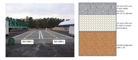
Fig. 2 Test pavement layout and pavement cross-section
