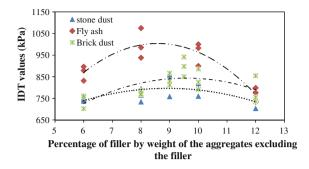
Fig. 2 Variation of IDT with varying percentage of filler (by weight of the aggregates excluding the filler) for stone dust, fly ash and brick dust
