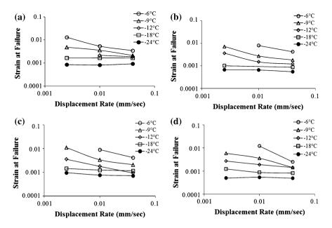
Fig. 3 Failure strain versus real deformation rate for **a** neat asphalt binder **b** 20 % BV1 asphalt mastic **c** 20 % CSG asphalt mastic and **d** 20 % HL asphalt mastic
