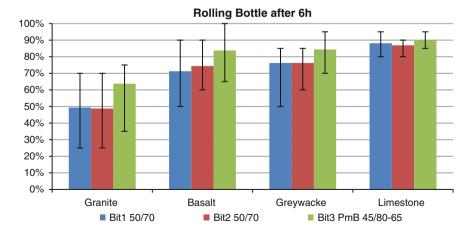
Fig. 1 Results of the rolling bottle test after 6 h
