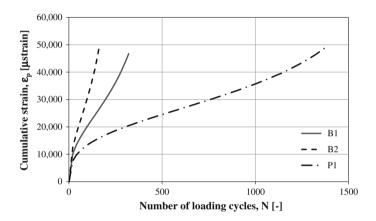
Fig. 4 Results of FN tests carried out at 58 °C on all bituminous mixtures
