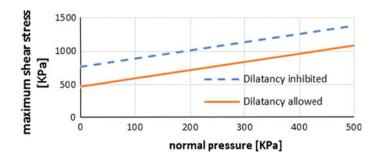
Fig. 8 Comparison of the results in the conditions of allowed or inhibited dilatancy
