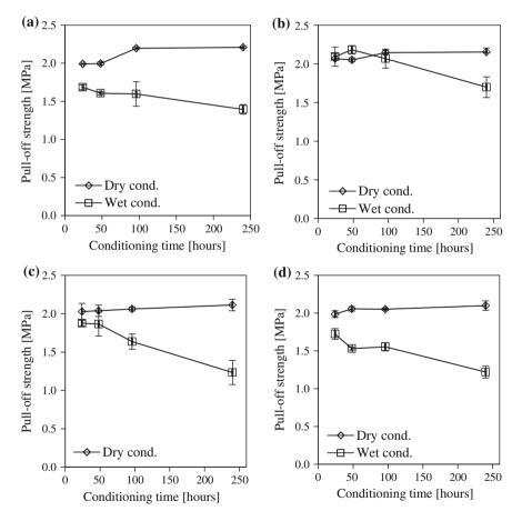
Fig. 4 Influence of conditioning and time on the pull-off strength for the different substrates, A (a), B (b), C (c) and D (d)
