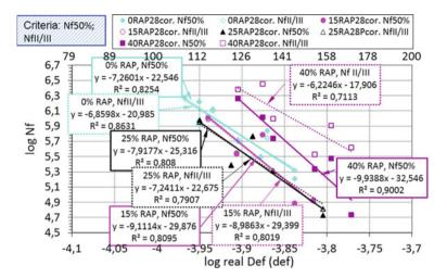
Fig. 4 Wöhler curves for the four mixes after correcting to air void of 5.1 % determined by the classical criterion and the criterion of the end of phase II
