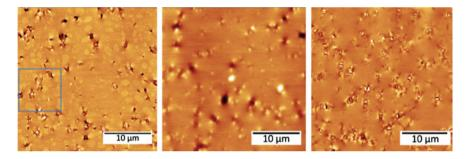
**Fig. 4** The original bitumen with an asphaltene content of 8.73 wt% (*left*, AFM topography scan of the maltene phase (*center*), and an artificially composed binder with an asphaltene content of 8.73 wt% (*right*) (Hofko et al. 2015)
