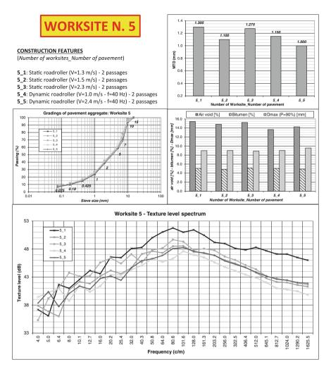
Fig. 2 Elaboration of the measurements carried out on the worksite n. 5
