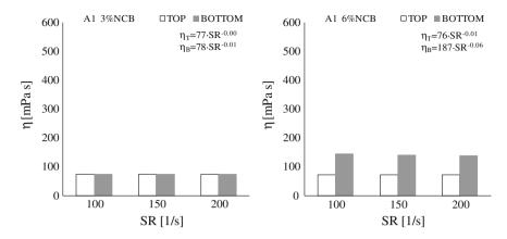
Fig. 4 Viscosity (n) versus shear rate (SR) of A1-NCB blends
