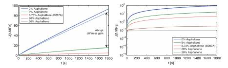
Fig. 3 Creep response of original and artificially composed bitumen samples from CR tests at +5 °C (Hofko et al. 2015)
