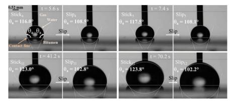
Fig. 6 Wetting behaviour of V70/100\_110\_cr\_fast during the dispensing of a 40  $\mu$ L-water drop using the dispensing rate of 0.2  $\mu$ L/s. Stick<sub>4</sub> and Slip<sub>4</sub> are the 4th stick and the 4th slip event, respectively; the stick event results in the maximum contact angle just before the slip event.  $\theta_a$  is the advancing contact angle which is calculated from the average between the contact angle on the right and the left sides of the water drop
