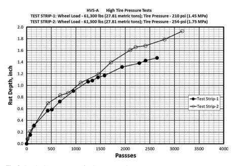
Fig. 8 Rut depth measurements for the two test strips
