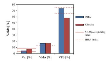
Fig. 9 Volumetric properties of the cores
