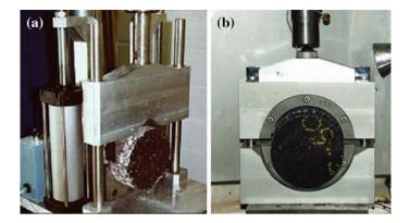
Fig. 1 a CH-LPDS shear device, b modified UK Leutner shear device
