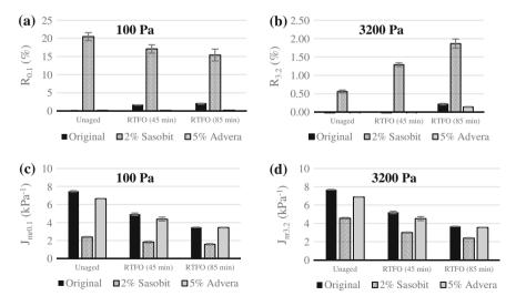
Fig. 6 MSCR results for unmodified 60/70 Pen binder mixed with WMA additives at different ageing processes: **a**  $R_{0.1}$  (%); **b**  $R_{3.2}$  (%); **c**  $J_{nr0.1}$  (kPa<sup>-1</sup>); **d**  $J_{nr3.2}$ (kPa<sup>-1</sup>)
