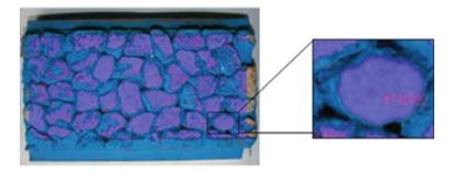
Fig. 7 Painted PSV test specimen with a selected aggregate using Image-Pro Plus
