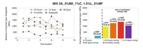
Fig. 2 Performance over time: mixture 2A
