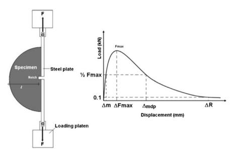
Fig. 1 Fenix test setup and load-displacement. Output curve (Pérez-Jiménez et al. 2010)
