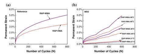
Fig. 3 Comparison of rutting resistance between RAP-HMA and RAP-WMA mixtures: a reference testing and b MSS testing conditions
