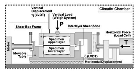
Fig. 1 Working scheme of ASTRA equipment
