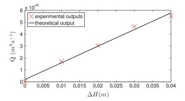
Fig. 5 Experimental outputs according to difference in load and associated line of linear regression
