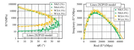
Fig. 4 Experimental results for tested materials: complex modulus in cole-cole axes; complex modulus in black diagram. 2S2P1D model was used to simulate data (Table 3)
