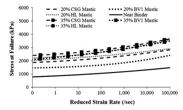
Fig. 5 Failure stress master curves for neat asphalt binder and asphalt mastics with 20 % filler
