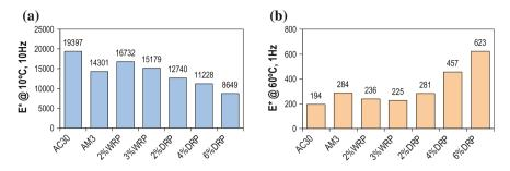
Fig. 4 Comparison of measured E\* a at 10 °C and 10 Hz, b at 60 °C and 1 Hz
