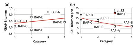
Fig. 8 Relationship between the RAP categorization and the asphaltic part of the RAP: **a** effect of the dosage of the bitumen on the RAP, and **b** effect of the penetration index (pene) measured on the recovery bitumen of the RAP
