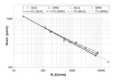
Fig. 4 Fatigue life N1 versus initial strain
