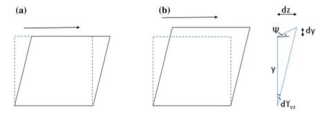
Fig. 1 Schematization of the shear test in inhibited (a) and allowed dilatancy (b)
