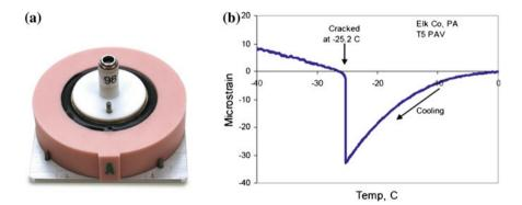
Fig. 1 Asphalt binder cracking device (ABCD): a ring and sample in a silicone mold; b a typical test results
