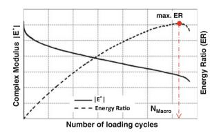
Fig. 3 Typical evolution of the complex modulus  $|E^*|$  and of the energy ratio (*ER*) over the number of loading cycles in a uniaxial tension-compression fatigue test
