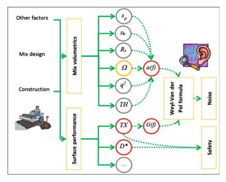
**Fig. 1** Graphical abstract of the paper. Legend  $s_{\rho}$ ,  $s_k$  viscous and thermal factors;  $R_s$  resistivity (Ns/m<sup>4</sup>);  $\Omega$  porosity;  $q^2$  tortuosity; *TH* thickness (mm); *TX* texture indicators; *G*(*f*) generation factors. (\*) *D* is considered a surface performance but it strongly depends on volumetrics
