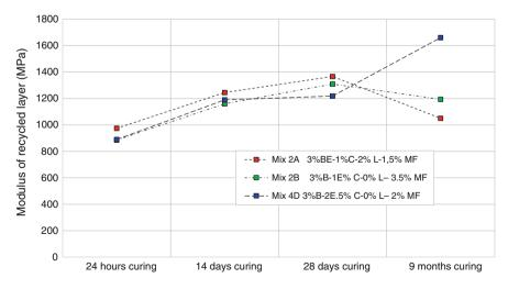
Fig. 5 Comparison of mixtures performance over time
