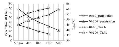
Fig. 1 Change in penetration and softening point in relation to the nr of hours of RCAT aging
