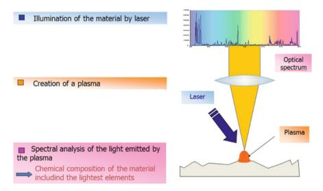
Fig. 2 The general principle of LIBS
