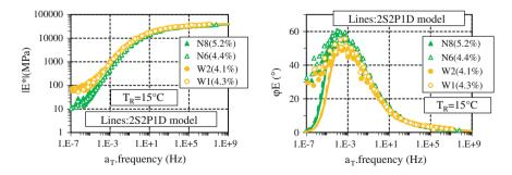
**Fig. 5** Experimental results for tested materials: master curves of the complex modulus (norm and phase angle). 2S2P1D model was used to simulate data (Table 3)
