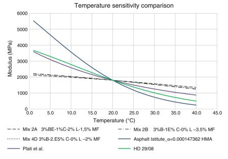
Fig. 1 Trend of moduli variation with temperature
