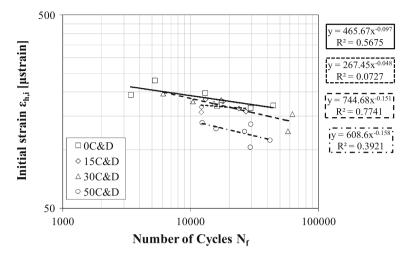
Fig. 5 Fatigue curve in terms of initial horizontal strain as a function of number of cycles
