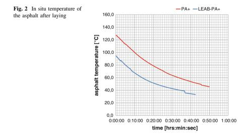
20–30 °C caused by lower production temperatures. Ageing of bitumen is mainly due to oxidation of the maltenes in the bitumen. The oxidation process is instigated by high temperatures and will result in a more stiff and less flexible bitumen. Based on the cooling curves, it is expected that the LEAB PA16+ mortar ageing is less extensive. Penetration tests on extracted bitumen or DSR tests on extracted mortar can confirm this statement. These tests will be discussed in the next paragraphs.
