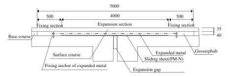
Fig. 1 Conventional embedded expansion joint
