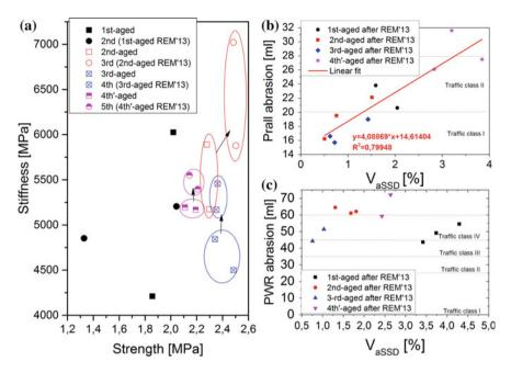
Fig. 2 a Relationship of strength and stiffness between different tested locations before and after REM'13; b relationship of Prall abrasion from the air voids measured by surface saturated dry method; c relationship of pavement wear resistance to studded tires (PWR abrasion) from the air voids measured by surface saturated dry method
