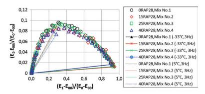
Fig. 3 Normalized complex modulus results for the mix tested
