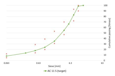
Fig. 1 Grading curve of AC 11 S (reference mixture)
