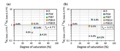
**Fig. 7** Relationship between the relaxation time established for a specific saturation state "i" ( $\tau_{0E,state}$ <sub>i,0 FTC</sub>), expressed relatively to the relaxation time obtained for the dry (D) sample ( $\tau_{0E,state}$  D,0 FTC), and the degree of saturation, before to apply any FT cycles (void content of samples indicated): **a** T<sub>0</sub> = 4.7 °C, **b** T<sub>0</sub> = -5.5 °C
