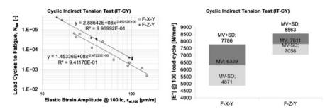
Fig. 3 IT-CY results: fatigue function (left), and stiffness (right)
