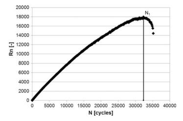
Fig. 3 Determination of failure  $N_1$  for mix S/LS at 0.9 MPa
