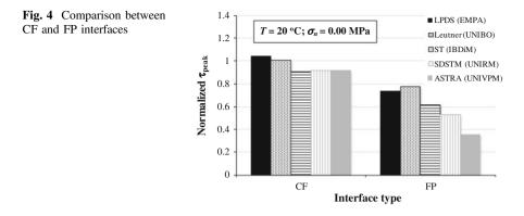
As far as the interlayer shear strength of the two interface types is concerned, whatever the experimental device and test conditions are, it is confirmed that FP geogrid produces a significant de-bonding effect with respect to the unreinforced interface, whereas CF geogrid results are very similar to those of UN interface.
