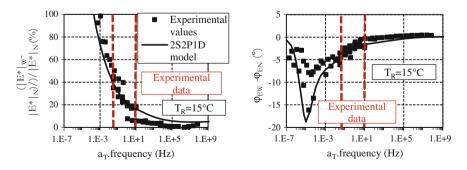
Fig. 9 Difference between the two types of mixtures with and without hydrated lime on the complex modulus (norm and phase angle)
