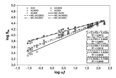
Fig. 3 Stiffness modulus master curves at 20 °C
