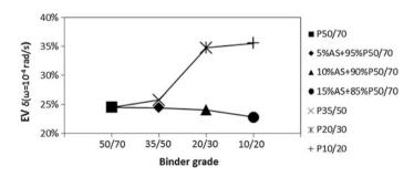
Fig. 7 Evolution of complex modulus phase angle after artificial ageing RTFOT and PAV
