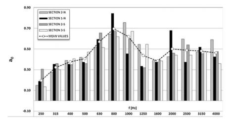
Fig. 2 Average acoustic absorption coefficients
