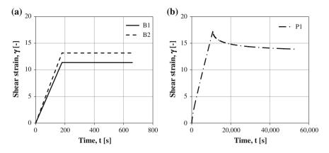
Fig. 1 Results of SSCR tests at 58 °C: a unmodified bitumens, b polymer-modified binder
