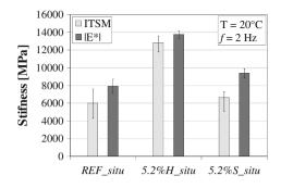
Fig. 4  $|E^*|$  and ITSM @ 20 °C and 2 Hz (equivalent to 124 ms rise time for ITSM) with the standard deviation error bars
