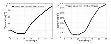
Fig. 3 Similar trend of the material temperature (a) and density (b) along the strip during the fifth pass of the roll
