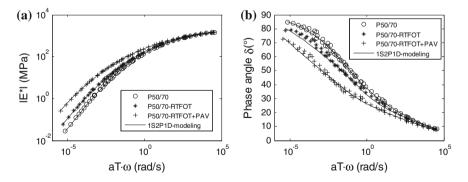
Fig. 1 a Complex modulus norm and **b** complex modulus phase angle master curves at  $T_{ref} = 0$  °C of a petroleum bitumen of grade 50/70 before and after artificial ageing procedures of RTFOT and PAV
