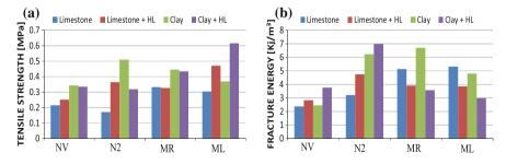
Fig. 5 Effect of filler on mastics tensile limits. a Tensile strength, b Fracture energy
