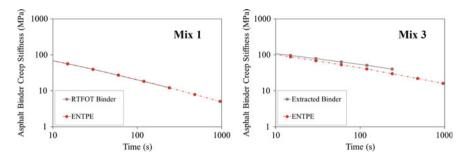
Fig. 3 Back-calculated and extracted creep stiffness of asphalt binder: mix 1 and 3
