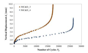
Fig. 2 Fatigue deformation storage curve of specimens containing 30 % and 50 % of C&D
