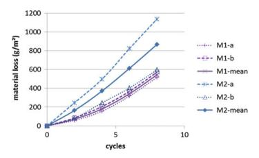
**Fig. 7** Test results for two variants of RUMG 6.3, at 20 °C (mix 1 has a higher binder content and is less discontinuous in grading than mix 2)
