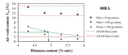
Fig. 2 Air voids content as a function of bitumen dosage for the 00RA mixture
