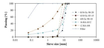
Fig. 1 Gradation of the aggregate fractions
