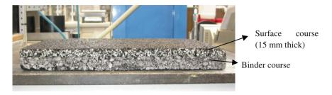
Fig. 6 Two-layered test plate with AC 14 binder course and RUMG 6.3 surface course
