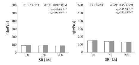
Fig. 8 Viscosity  $(\eta)$  versus shear rate (SR) of B1-CNT blends
