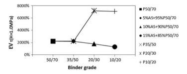
Fig. 9 Evolution of the relaxation time after artificial ageing RTFOT and PAV
