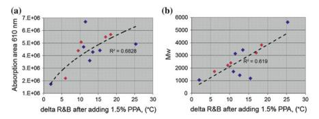
Fig. 4 Relation between the interaction with PPA and chemical characteristics of the binders: a relation to the uv-vis absorption area at 610 nm, b relation to Mw (B11 is not included)
