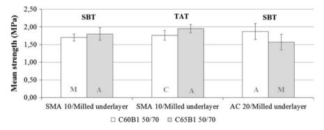
Fig. 2 Results of interlayer bonding tests (SBT, TAT)-Impact of tack coat type on milled underlayers. Note that the failure modes are indicated in each bar (A adhesion, C cohesion, M mixed). The *error bars* represent the standard deviation
