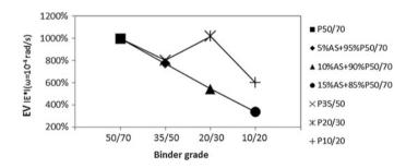
Fig. 6 Evolution of complex modulus norm after artificial ageing RTFOT and PAV
