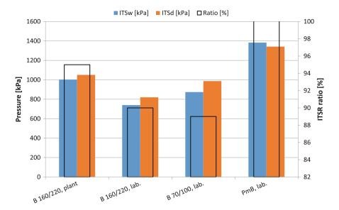
Fig. 5 Water sensitivity (ITSR)—AC 11 S 40 % RAP (reference virgin aggregates)
