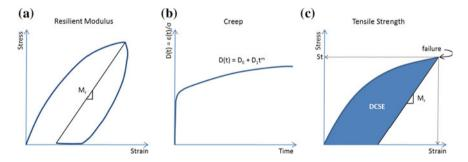
Fig. 2 Parameters determined from a resilient modulus, b creep, and c strength tests
