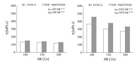
Fig. 2 Viscosity (n) versus shear rate (SR) of B1-NCA blends
