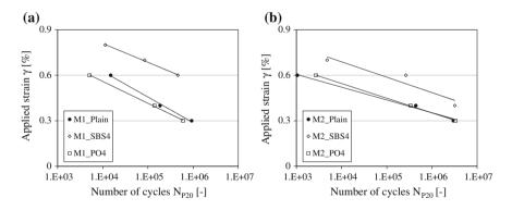
Fig. 3 Fatigue curves in terms of N<sub>P20</sub>: a Mastics M1. b Mastics M2
