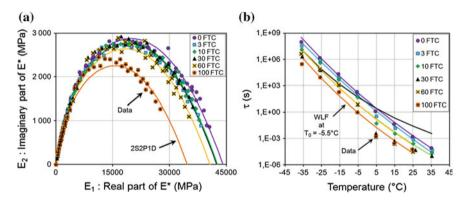
Fig. 5  $E^*$  results in accordance with FTC of the PSW sample: **a** cole-cole plane, **b** relationship between the relaxation time and the  $E^*$  testing temperatures
