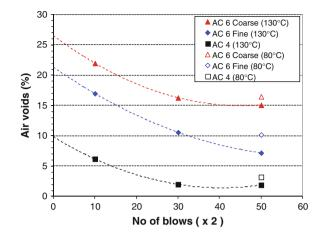
**Fig. 2** Effect of compaction effort and compaction temperature on air voids
