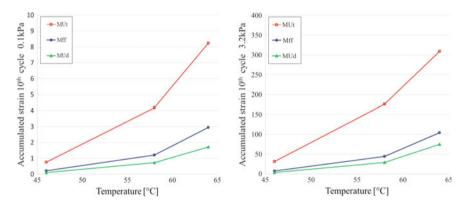
Fig. 7 Accumulated strain values at the end of 10th cycle at 0.1 and 3.2 kPa
