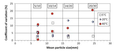
Fig. 5 Relationship between the coefficient of variation values (CV%) and the mean particle size of fraction group tested at different temperatures
