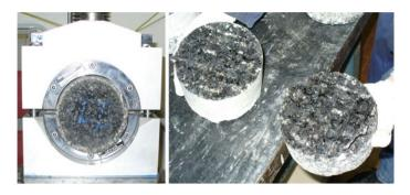
Fig. 7 Leutner shear testing and a tested specimen
