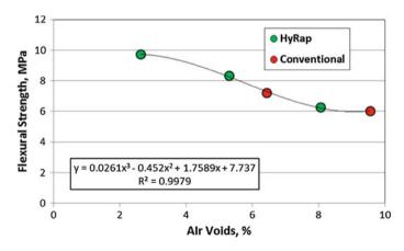
Fig. 6 Relationship between air voids and flexural strength
