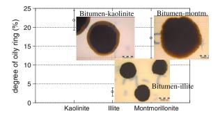
Fig. 2 Screenshots of bitumen-clay spots and calculated degree of Oliensis (ratio of the oil ring to whole spot radii)
