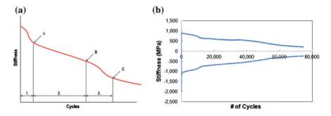
Fig. 2 a General behavior of NBF stiffness. b Example of real stiffness data
