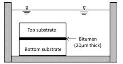
Fig. 3 Specimen of aggregate-bitumen bond submerged into water
