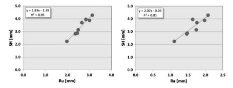
Fig. 4 Ru and Ra versus sand height
