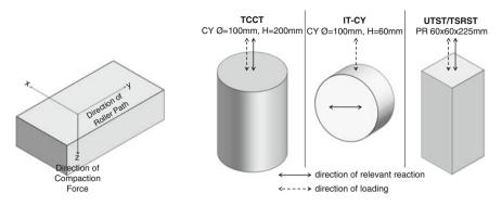
Fig. 1 Coordinate system of compaction (left) and principal directions of testing (right)
