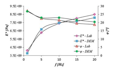
Fig. 7 2nd set of variable Burger's contact model, compared with lab test data
