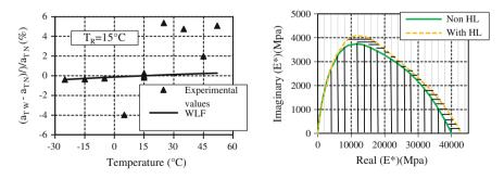
Fig. 11 Difference between the two types of mixtures with and without hydrated lime on the shift factors  $a_T$  (*left*) and on the area of cole-cole curves (*right*)
