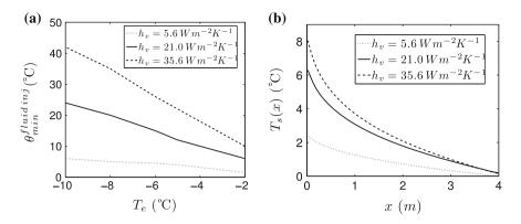
**Fig. 8** a Evolution of minimum fluid injection temperature with outside temperature for  $h_v = 5.6$ , 21, and  $36.5 \text{ Wm}^{-2}\text{K}^{-1}$  for abscissa L = 4 m and **b** profile of surface temperature with fluid circulation for different values of  $h_v$  and  $T_e = -10$  °C.
