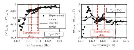
Fig. 10 Difference between the two types of mixtures with and without hydrated lime on the Poisson's ration "average" (norm and phase angle)
