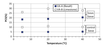
Fig. 6 Relationship between the percentage passing through the control sieve (PSC%) of fragmentation tests done on the 5/10 mm fraction group of two different sources of virgin aggregates (VA) and the testing temperature measurements
