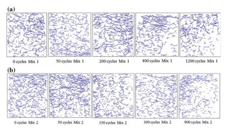
Fig. 7 Evolve in aggregate skeleton connectivity during loading: a mix 1, b mix 2
