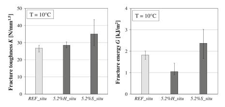
Fig. 5 Semi-circular bending test results: fracture toughness K (left); fracture energy G (right)
