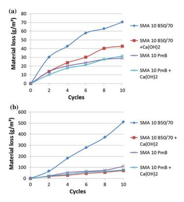
Fig. 3 Test results for SMA 10 showing impact of binder type and use of Ca(OH)<sub>2</sub>: **a** at 27 °C, **b** at 40 °C
