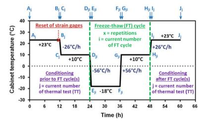
**Fig. 3** Cabinet temperature history during thermal test sequence (TT): "j" is the current number of TT (Fig. 1) and "i" is the current number of freeze-thaw (FT) cycles (Lamothe et al. 2014)
