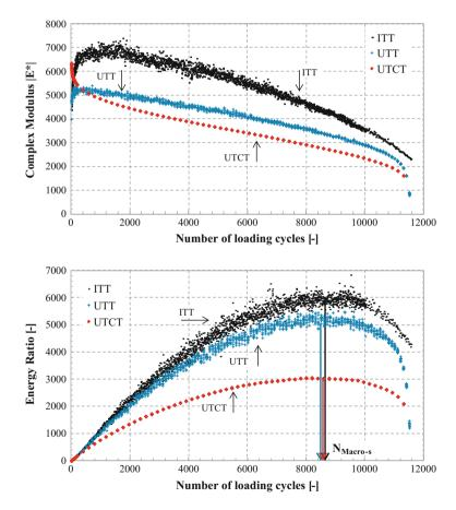
Fig. 6 Evolution of absolute value of complex modulus and energy ratio over the number of loading cycles and achieved  $N_{Macros}$  in indirect tensile test (ITT), uniaxial tension test (UTT) and uniaxial tension-compression test (UTCT)
