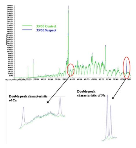
Fig. 9 Spectra of the 2 bitumens
