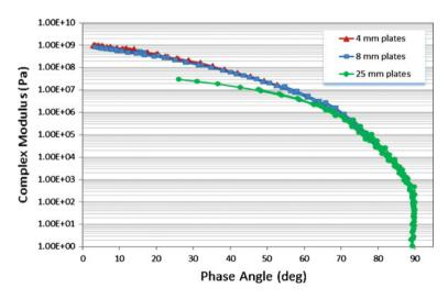
Fig. 2 Examples of complex modulus versus phase angle obtained by parallel plates of different diameters (sample B)
