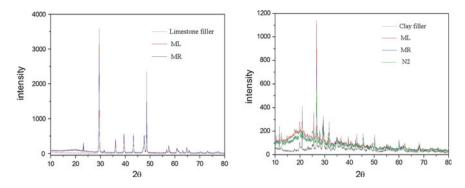
Fig. 8 Diffraction patterns for the mastics and the related filler
