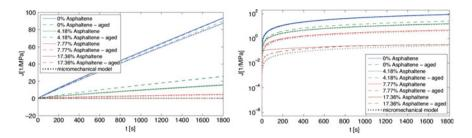
**Fig. 6** Comparison of experimental results and multiscale model predictions for aged artificial bitumen with asphaltene contents of 4.18, 7.77, 12.32 and 17.36 % at +5 °C. Creep compliance is shown on a linear scale (*left*) and on a logarithmic scale (*right*) for a better representation of creep curves with high asphaltene content
