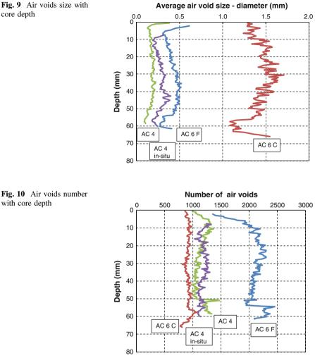
Fig. 10 Air voids number with core depth
