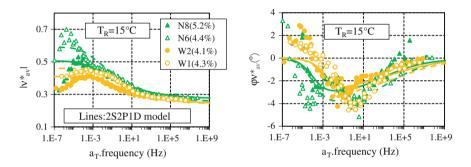
Fig. 7 Master curves of the Poisson's ration "average" (norm and phase angle). 2S2P1D model was used to simulate data (Table 3)
