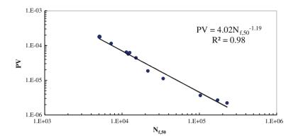
Fig. 4 PV versus N<sub>f,50</sub> plot for all tested binders
