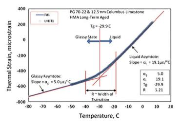
Fig. 3 Comparison of the Bahia and Anderson equation fit versus the data for the PG 72-22 binder, limestone aggregate mix
