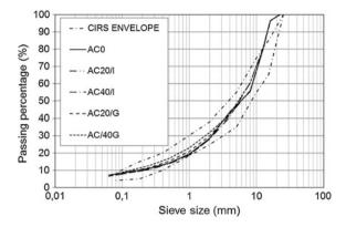
Fig. 2 Grading curves of the mixes
