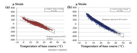
Fig. 11 Results of static strain at road shoulder: a new joint method, b conventional joint method
