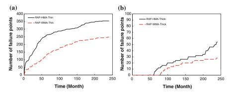
Fig. 4 Fatigue life prediction for: a thin pavement and b thick pavement
