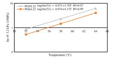
Fig. 5 Results of MSCR test and fitted model for two asphalt binders
