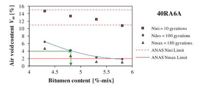
Fig. 4 Air voids content as a function of bitumen dosage for the 40RA6A mixture
