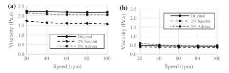
**Fig. 7** Viscosity measurement at different rotational speed for **a** modified PG 76-22 asphalt binder and **b** unmodified 60/70 Pen asphalt binder mixed with WMA additives
