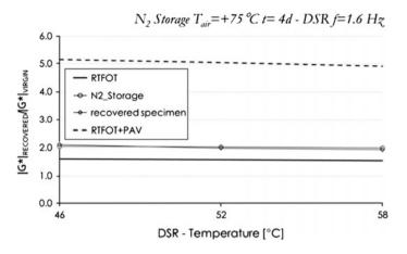
Fig. 3 Change in dynamic shear modulus  $|G^*|$  of bitumen recovered from  $N_2$  stored HMA specimen to virgin bitumen sample
