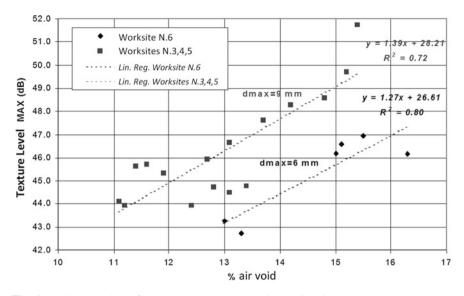
Fig. 6 Maximum values of the texture levels versus mixture air void contents
