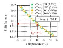
**Fig. 6** Shift factors  $a_T$  identical for E\* and v\* of the tested materials and WLF fitting law (Eq. 9) (constants given in Table 3)
