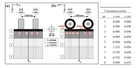
Fig. 3 Pavement model with A330-300 loads: a x-z view, b y-z view and calculation points
