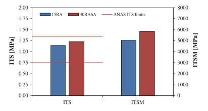
Fig. 10 ITS and ITSM values of the cores
