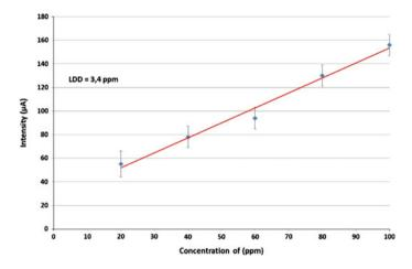
Fig. 7 Calibration line for Ni with the monochromator
