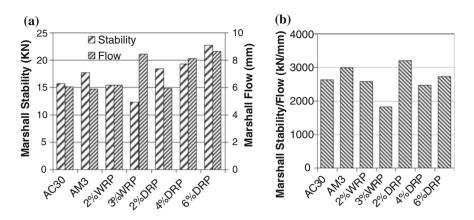
Fig. 1 Marshall test results: a Stability and flow. b Marshall quotient
