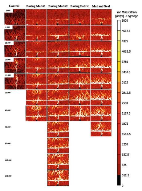
Fig. 1 Crack propagation in the NBF test
