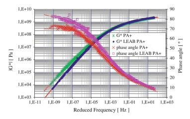
Fig. 3 Shear modulus mastercurve at -10 °C of LEAB-PA16+ and standard PA16+ after production; highway A18 test section
