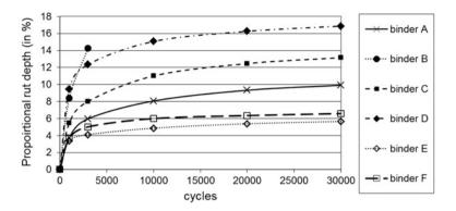
Fig. 2 Overview of the wheel tracking test for a series of coloured AC6.3 mixtures
