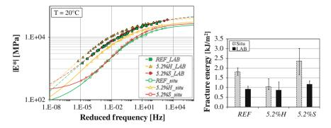
Fig. 7 Laboratory versus field mixtures: stiffness values (left); fracture energy (right)
