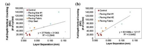
Fig. 3 Correlation between layer separation and cycles to full depth cracking: **a** including chip seals and **b** geosynthetics and control samples only
