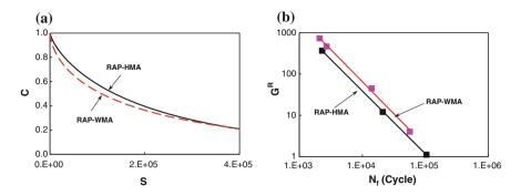
Fig. 2 Comparison of: **a** fitted damage characteristic curves and **b** failure criterion lines for the study mixtures
