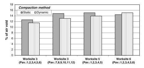
Fig. 4 Comparison between pavement air void contents resulting from dynamic and static compaction
