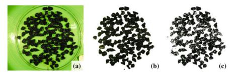
Fig. 2 Image filtering process. a Original image; b Non-classified image; c Classified image
