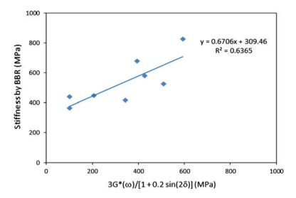
Fig. 8 Correlation between 4-mm DSR at 0.0167 rad/s estimated from master curves at a reference temperature of -25 °C and BBR stiffness measured at the same temperature
