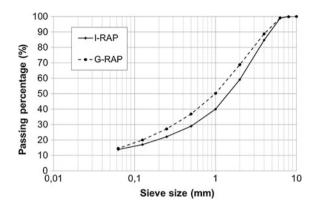
Fig. 1 Grading curves of the RAP aggregates
