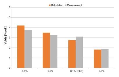
Fig. 3 Mix design optimization: void content calculation (AC 11 S, 40 % RAP, B160/220)
