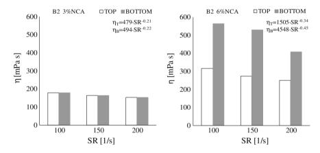
Fig. 3 Viscosity  $(\eta)$  versus shear rate (SR) of B2-NCA blends
