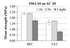
Fig. 5 Results of interlayer bonding tests (SBS, TAT)-Impact of curing time. The *error bars* represent the standard deviation
