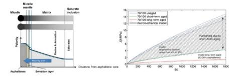
**Fig. 7** Model for the polarity distribution in material phases, for unaged (*black line*) and aged (*blue line*) bitumen (*left*), and comparison of experimental results and micromechanical model predictions for unaged, RTFOT– and RTFOT+PAV-aged natural bitumen pen 70/100 (*right*)
