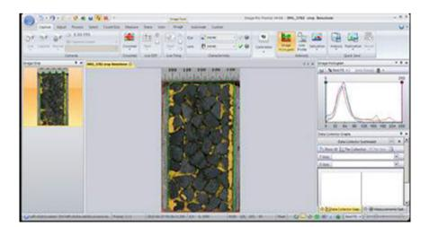
Fig. 4 Image-Pro analysis of PSV test specimen to determine contact with tyre (McCall 2013)
