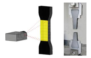
Fig. 4 Mastic modified direct tension test configuration
