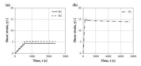
Fig. 2 Results of SSCR tests: a unmodified bitumens at 46 °C, b polymer-modified binder at 76 °C
