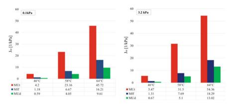
Fig. 8 Mff, MUt and MUd non recoverable compliance at 0.1 and 3.2 kPa
