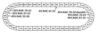
Fig. 1 Layout of the test sections on NCAT pavement test track
