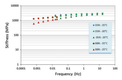
Fig. 7 Stiffness moduli calculated from G\* by 4-mm DSR or measured by BBR (sample B)
