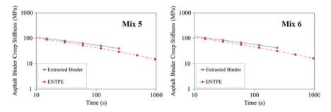
Fig. 4 Back-calculated and extracted creep stiffness of asphalt binder: mix 5 and 6
