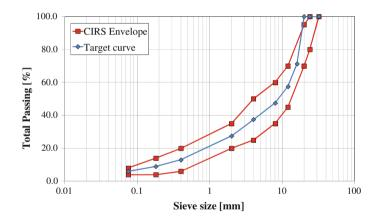
Fig. 1 Gradation curve of the aggregate blend
