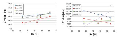
Fig. 2 Results of DSR at 60 and 25 °C in function of filler RVs
