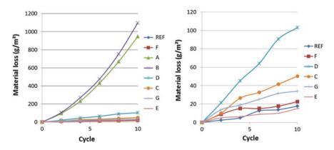
Fig. 8 Loss of material in the raveling tester at 20 °C (the two graphs are the same, except for the scaling of the vertical axis)
