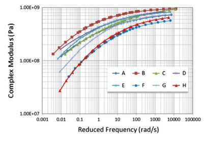
Fig. 4 Master curves at reference temperature of -25 °C
