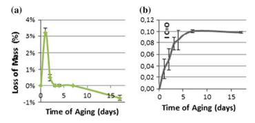
Fig. 1 a Mass loss % from 0–17 days of bitumen aging. b Change in  $I_{C=0}$  0–17 days for bitumen oven aging (average of three samples)
