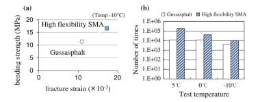
Fig. 5 Test results: **a** bending strength and fracture of strain by bending strength test at -10 °C, **b** bended fatigue test results
