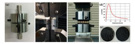
Fig. 4 Procedures for bonding strength evaluation
