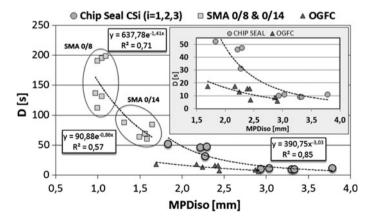
Fig. 6 Drainability (y-axis) versus macrotexture (x-axis)
