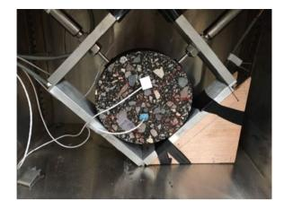
strain gauge instrumented inside of the ring detects this fracture. A typical ABCD test result is shown in Fig. 1b.
