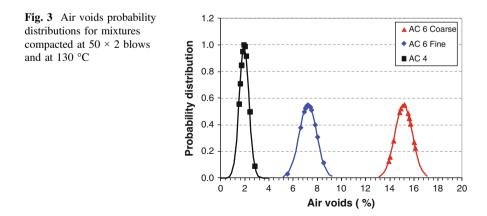
determined were  $15.1 \pm 0.6$  % for the AC 6 Coarse,  $7.2 \pm 0.6$  % for the AC 6 Fine and  $1.9 \pm 0.3$  % for the AC 4 mixture. Thus, less variability in the air void content was determined for the AC 4 mixture.
