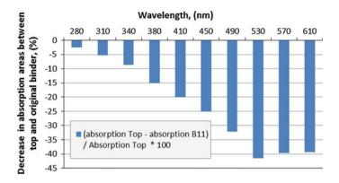
Fig. 8 Change in uv-vis absorption areas for B11 between B11 and the top part of B11 + 3 % PPA
