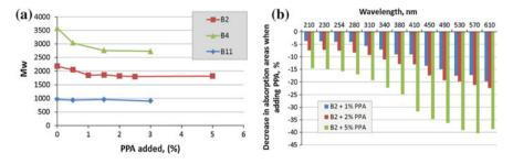
Fig. 3 Changes in the GPC measurements after adding PPA **a** changes in Mw, **b** changes in the uv-vis absorption areas
