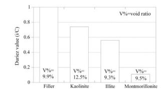
same proportion of clay (9 %), the water resistance drop varies with clay mineralogy, and the kaolinite-rich AC mixtures being less affected than illite-rich and far less than montmorillonite-rich AC mixtures.
