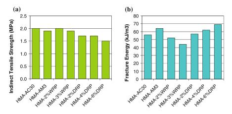
Fig. 2 a Indirect tensile strength. b Fracture energy for the seven mixtures
