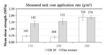
Fig. 4 Results of shear bond test-Impact of tack coat application rate and nature and preparation of the underlayer for the interface between AC 20 and two underlayers. Note that the measured tack coat rates are indicated above each bar. The *error bars* represent the standard deviation
