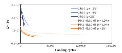
Fig. 1 G\* evolution for the 35/50 bitumen with different strain levels
