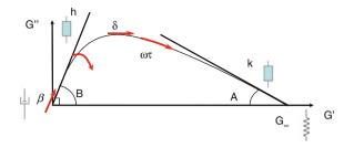
Fig. 5 Cole-Cole diagram of parameters influence with ageing
