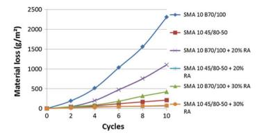
Fig. 4 Test results for SMA 10 (different binders and use of reclaimed asphalt), at 40 °C
