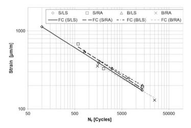
Fig. 2 Fatigue life N<sub>f</sub> versus initial strain
