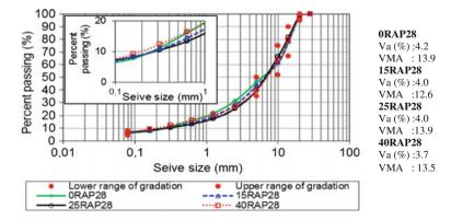
Fig. 1 Asphalt mixtures gradations and characteristics
