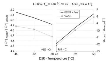
Fig. 6 Change in dynamic shear modulus  $|G^*|$  (*left*) and phase angle  $\varphi$  (*right*) of bitumen recovered from VAPro-aged HMA specimen to virgin bitumen sample
