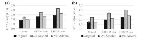
**Fig. 3** Rutting factor  $(G^*/\sin(\delta))$  for **a** modified PG 76-22 binder at 76 °C and **b** unmodified 60/70 Pen binder at 64 °C mixed with WMA additives at different ageing processes
