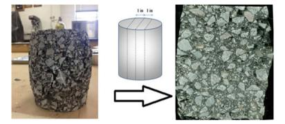
Fig. 5 Cutting section of a failed sample
