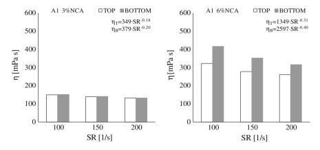
Fig. 1 Viscosity ( $\eta$ ) versus shear rate (SR) of A1-NCA blends
