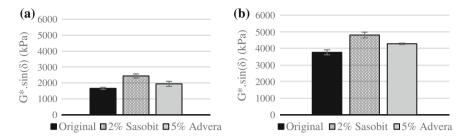
**Fig. 4** Fatigue Factor ( $G^* \cdot \sin(\delta)$ ) for **a** modified PG 76-22 binder at 31 °C and **b** unmodified 60/70 Pen binder at 25 °C with different WMA additives and aged by PAV system for long-term ageing
