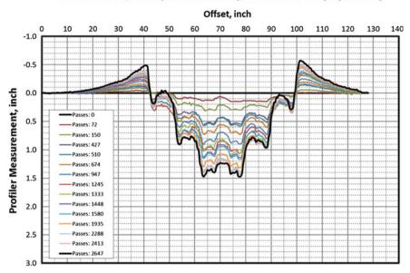
HVS-A High Tire Pressure Tests TEST STRIP-1 Wheel Load - 61,300 lbs (27.91 metric tons); Tire Pressure - 210 psi (1.45 MPa)
