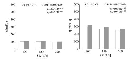
Fig. 9 Viscosity  $(\eta)$  versus shear rate (SR) of B2-CNT blends
