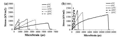
Fig. 2 Effect of temperature on stress-strain curves for **a** neat asphalt binder **b** 20 % HL asphalt mastic
