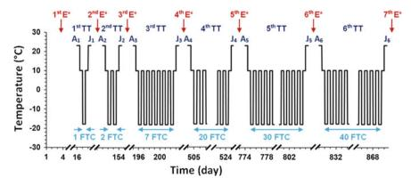
Fig. 1 Six thermal test (TT) sequences of freeze-thaw cycles (FTC) applied to the samples
