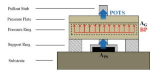
**Fig. 1** Bitumen bond strength test: schematic representation of the test. The different components used to evaluate the pull off tensile strength (POTS) are highlighted: the contact area between the gasket and the pressure plate  $(A_G)$ ; the burst pressure (BP) and the area of the pull off stub  $(A_{PS})$
