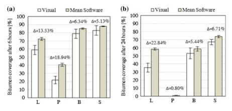
Fig. 3 Results of rolling bottle tests after 6 h (a) and 24 h testing (b)
