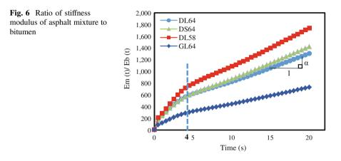
aggregate structure. The aggregate structure factor (ASF) composed of aggregate geometric properties, contact points and lengths, as shown in "Eq. 14", was introduced to describe the aggregate microstructure. Figure 6 shows that two linear segments exist in the plot of stiffness ratios with time. "Equation 15" describes this relationship.
