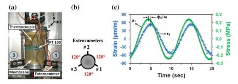
Fig. 4 Setup used to measure  $E^*$ : a specimen and measurement system, b top view, c example of stress-strain measurements and sinusoidal fitting curves (f = 0.1 Hz and T = 15 °C)
