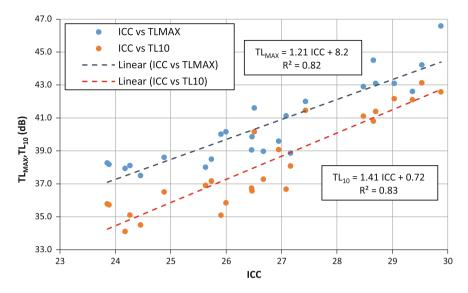
Fig. 7 Regression between index of the composition of the wearing course and texture levels
