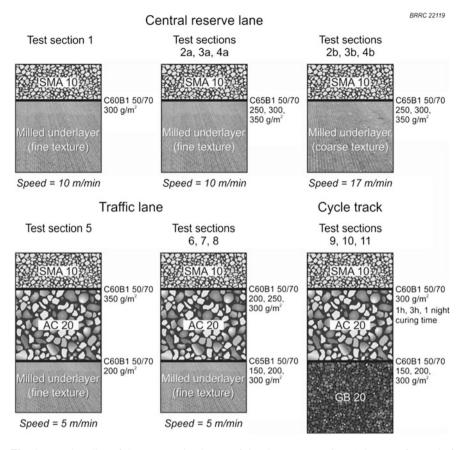
Fig. 1 Broad outline of the construction layout of the eleven test sections (The rate of spread of emulsion is expressed in target residual binder quantities in  $g/m^2$ )
