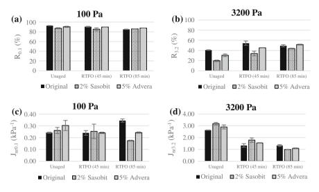
Fig. 5 MSCR results for modified PG 76-22 binder mixed with WMA additives at different ageing processes: **a**  $R_{0,1}$  (%); **b**  $R_{3,2}$  (%); **c**  $J_{nr0,1}$  (kPa<sup>-1</sup>); **d**  $J_{nr3,2}$ (kPa<sup>-1</sup>)
