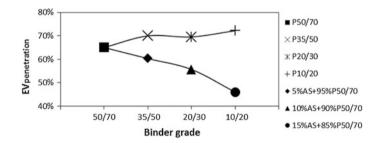
Fig. 4 Evolution of penetration after artificial ageing RTFOT and PAV
