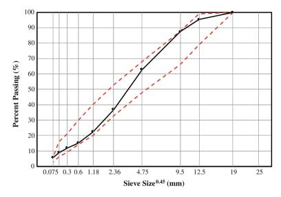
Fig. 4 Job mix formula gradation (dashed lines represent FAA P-401 gradations limits)
