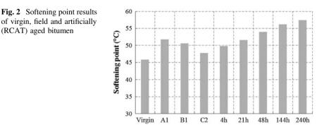
service life of B1 is 11 years, a higher softening point is expected than A1, which has a service life of 5 years. Possibly the short term ageing caused by production, transport and laying may differ, but this is unknown. The results suggest that to mimic 5–11 year field ageing of the bitumen of the top layer, it takes about 21 h artificial ageing with RCAT to obtain identical softening points while for the binder layer, it takes less than 4 h.
