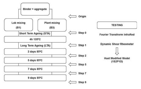
Fig. 1 Resume of the experimental design
