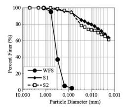
Fig. 1 Particle size distribution curves of collected materials
