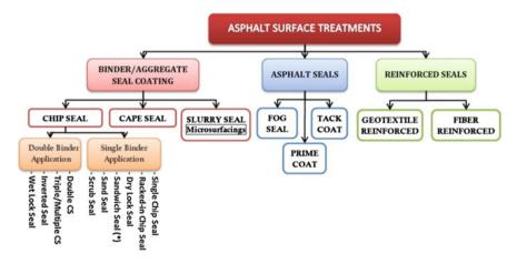
Fig. 1 The most common solutions for asphalt surface treatments. *Note CS* chip seal; \* single/double chipping
