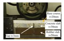
Fig. 4 Penetration with crack test by wheel load
