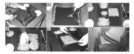
**Fig. 3** Construction phases: **a**, **b** emulsion spraying on the support layer (after storing in the oven at a temperature of  $69 \pm 2$  °C); **c**, **d** application of a uniform layer of clean limestone aggregates; **e** a rubber sheath is laid on the surface in order to avoid the crushing of the aggregate during compaction; **f** slab compaction by means of the Unical Slab Roller Compactor (USRC) (Praticò and Vaiana 2013) (UNI EN 12697-33)
