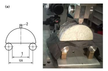
Fig. 4 a Monotonic semi-circular bending test and b experimental setup with coated specimen
