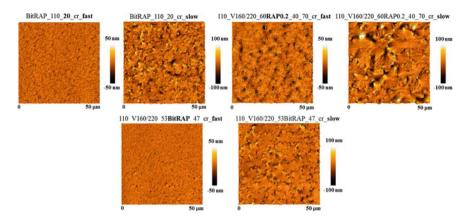
Fig. 4 AFM topography images of the surface of different films. Scan area is  $50 \times 50 \ \mu m^2$
