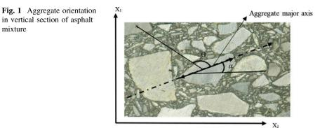
orientation of an asphalt mixture. The value of  $\Delta$  ranges from zero to unity. A zero value denotes complete random distribution of aggregates, which is analogous to an isotropic material, and unity denotes aggregates oriented in only one direction and is analogous to an anisotropic material.
