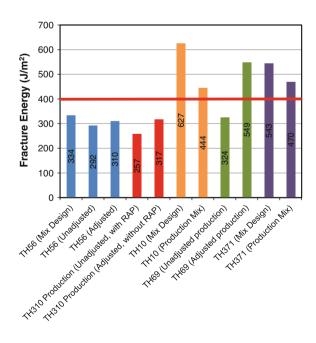
Fig. 4 Summary of DCT pilot study testing
