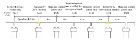
Fig. 8 Location in test operation: P446 was repaired by new method, P450 was repaired by conventional method
