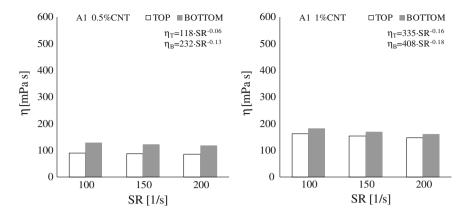
Fig. 7 Viscosity  $(\eta)$  versus shear rate (SR) of A1-CNT blends
