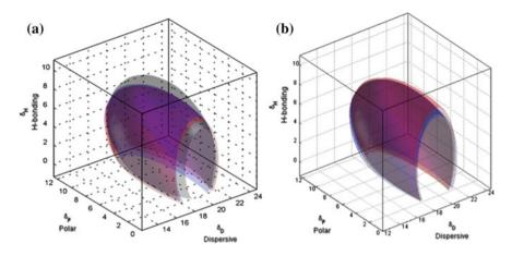
**Fig. 3** a Solubility parameters of recovered bitumens 2nd site (*red*), 3rd site (*blue*) and 4th site (*black*) indicating minuscule changes in solubility between the materials; **b** an example of soft bitumens solubility parameter (*red*) with bitumens from 3rd site (*blue*) and 4th site (*black*)
