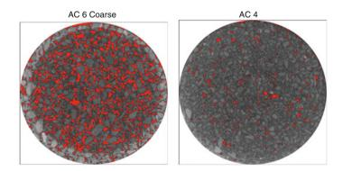
Fig. 7 CT scans (mid height of the core—air voids in red)
