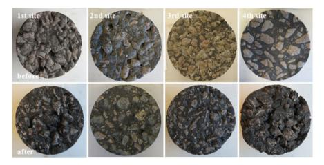
Fig. 1 The cores from HW1 taken from locations (1, 2, 3 and 4) representative of different aging cycles of life before (*upper row*) and after REM'13 treatment (*lower row*)
