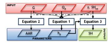
**Fig. 5** Closed-form Eqs. (1–3) to design a surface treatment based on surface properties. *Symbols G* aggregate grading; *z* bitumen film thickness;  $h_B$  Bitumen height; *AAR* aggregate application rate, g/cm<sup>2</sup>;  $Q_B$  quantity of bitumen per square meter, g/m<sup>2</sup>;  $SH_{int}$  sand height of the underneath layer; *SH* sand height of the upper layer
