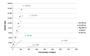
Fig. 6 Calibration lines for the various elements
