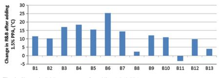
Fig. 1 Change in R&B temperature after adding 1.5 % PPA
