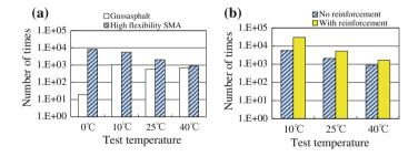
Fig. 6 Test results: a penetration with crack test results, b compared with the effect of rein forcing material
