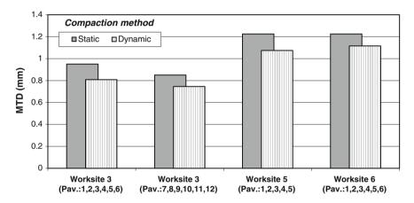
Fig. 5 Comparison between MTD measured on pavement with dynamic and static compaction
