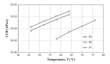
Fig. 3 CCR values as a function of test temperature
