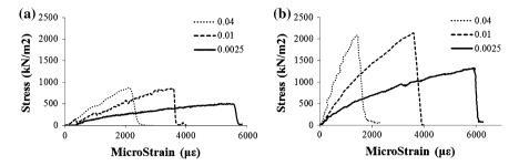
Fig. 1 Effect of deformation rate on stress-strain curves for **a** neat asphalt binder **b** 20 % HL asphalt mastic
