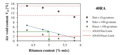
Fig. 3 Air voids content as a function of bitumen dosage for the 40RA mixture
