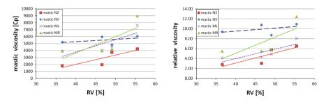
Fig. 1 Influence of RV on mastic viscosity and relative viscosity
