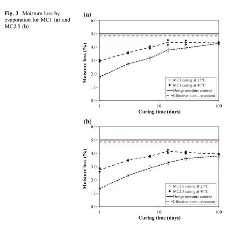
Analogously, for mixture MC2.5, the moisture loss after one day curing was 2.6 and 1.4 % at 40 and 25 °C, respectively. This difference reduced at longer times and at 100 days, the same weight loss (3.9 %), was measured for both curing temperatures. In addition, it can be observed that, at 40 °C, the moisture loss did not increase after 14 days anymore, whereas at 25 °C such an "equilibrium" condition was not obtained before 100 days.
