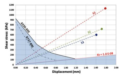
Fig. 8 Stress-displacement graph: comparison between tests and models results
