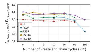
Fig. 9 Relationship between the evolution of the glassy modulus established for each saturation state "i" ( $E_{0,state\ i,0\ FTC}$ ) expressed relatively to the glassy modulus of the tested dry sample before to be submit to FTC
