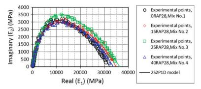
Fig. 2 Complex modulus results in Cole-Cole plan and 2S2P1D and WLF parameters
