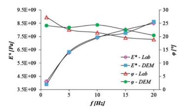
Fig. 5 Constant Burger's contact model compared with lab test data
