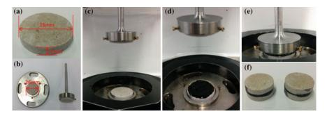
Fig. 2 Aggregate-bitumen sample preparation procedures
