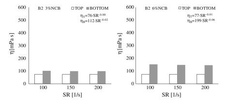
Fig. 6 Viscosity (n) versus shear rate (SR) of B2-NCB blends
