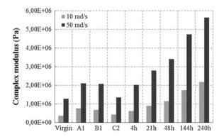
describe the measured data within the tested range. The found differences for the model parameters indicate that due to ageing, the response of the different bitumens at a given temperature changes. This is illustrated in Fig. 3.
