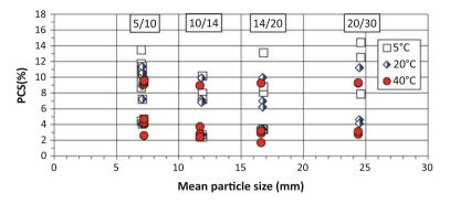
Fig. 4 Relationship between the PCS% of RAP sources tested and the mean particle size of fraction groups tested at different testing temperatures
