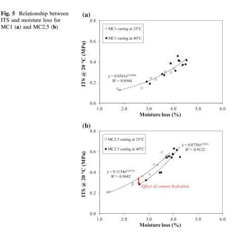
cement, the curing level measured by ITS resulted from the combined effect of both moisture loss by evaporation and cement hydration.
