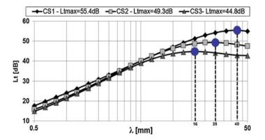
Fig. 7 Maximum texture level and texture wavelength versus aggregate dimension
