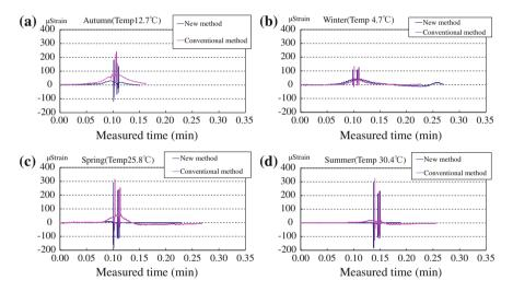
**Fig. 12** Results of dynamic strain on the base course in site: **a** results in the autumn (12 November 2013), **b** results in the winter (17 February 2014), **c** results in spring (16 June 2014), **d** results in summer (19 August 2014)
