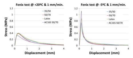
Fig. 3 Load displacement curves obtained in the Fenix tests performed at +20 and -5 °C
