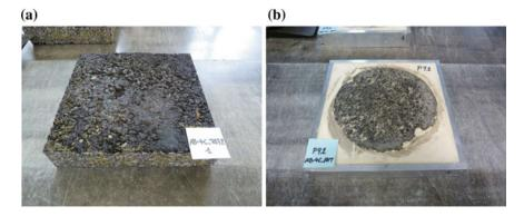
Fig. 2 a Test plate compacted in the lab. b Test core from a road, cast in a test mould
