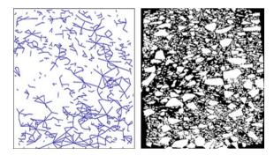
Fig. 8 Discontinuity of aggregate structure at outer layers due to bulging represented by *black* and *white* image and aggregate skeleton network
