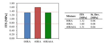
Fig. 5 ITS on specimens compacted under 100 gyrations, comparison with Italian specifications
