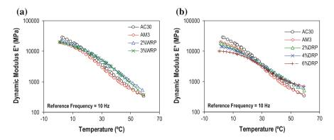
Fig. 3 Variation of  $E^*$  as a function of the temperature for the mixtures containing RP **a** added by the wet process, **b** added by the dry process
