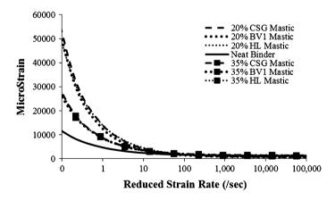
Fig. 4 Failure strain master curves for neat asphalt binder and asphalt mastics with 20 and 35 % filler
