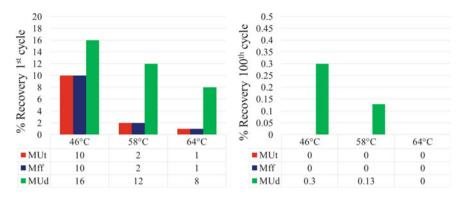
Fig. 5 Comparison of RCR percentage recovery at the 1st and 100th cycle @ 46, 58 and 64 °C
