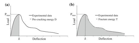
Fig. 3 Analysis of 3PB test results: a pre-cracking energy D, b fracture energy T
