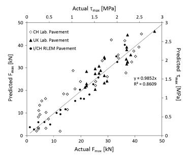
Fig. 3 Prediction of  $F_{max}$  and  $\tau_{max}$  for the independent query test dataset
