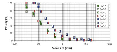
Fig. 1 Grading curve of RA (black curve)
