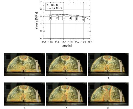
Fig. 7 Crack propagation in a monotonic bending test (AC 8 D S)
