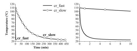
**Fig. 1** Profiles of the cooling rates cr\_fast and cr\_slow for V70/100 using annealing temperature of 110 °C. The plot on the *right* shows a close-up of the profiles for the first 10 min
