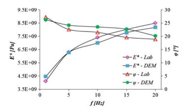
Fig. 6 1st set of variable Burger's contact model, compared with lab test data
