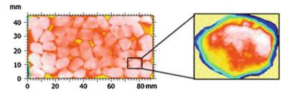
Fig. 8 Colour depth classified painted PSV test specimen 3d model with form removed showing selected area particle using MountainsMap 7
