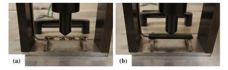
Fig. 1 Bending beam rheometer with thin a asphalt mixture and b asphalt binder beams
