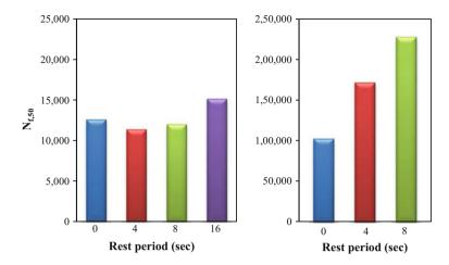
Fig. 3 Effect of rest periods on fatigue life
