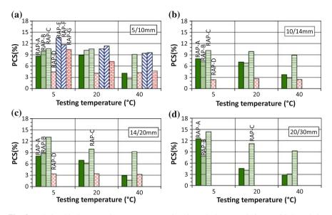
Fig. 3 Relationship between the percentage passing through the control sieve (PCS%) and the fragmentation testing temperature on different RAP sources: **a** fraction group—5/10 mm, **b** fraction group—10/14 mm, **c** fraction group—14/20 mm, **d** fraction group—20/30 mm
