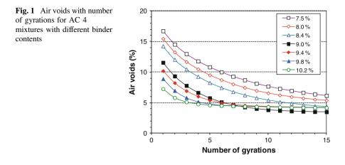
Based on the above the target binder content selected for the AC 4 mixture was 9.0 %. Thus, the designed binder content of the AC 4 mixture was higher than those of the AC 6 mixtures. Also, the grading of the AC 4 mixture was finer than those for the AC 6 mixtures (see Table 1).
