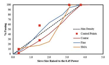
Fig. 2 Gradations of mixtures
