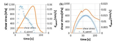
Fig. 6 Dilatancy speed in the SISTM (a) and dilatancy speed in the SDSTM (b)
