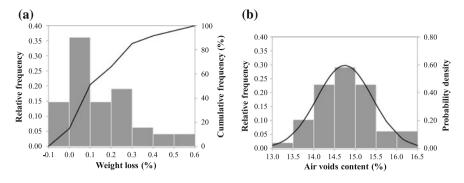
Fig. 2 Relative frequency distribution of the measurements of weight loss (a) and air voids content  $V_m$  (b)
