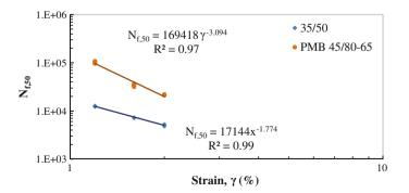
Fig. 2 Traditional N<sub>f.50</sub>—strain relationship for bitumen's fatigue testing results
