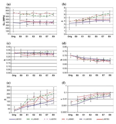
Fig. 4  $G_{\infty}$ ,  $\delta$ , k, h,  $\beta$  and  $\tau$  laboratory and plant mixtures modelling results
