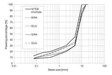
Fig. 1 Grading curves of the mixes
