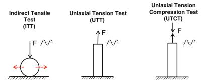
Fig. 2 Principles of the indirect tensile test (*left*), uniaxial tension test (*middle*) and uniaxial tension compression test (*right*)
