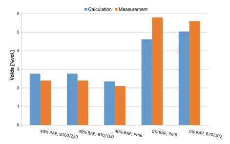
Fig. 2 Difference between calculations and measurements for reference AC 11 S (6.10 % binder)
