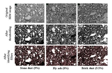
Fig. 6 Images at optimum filler contents for stone dust, fly ash and brick dust
