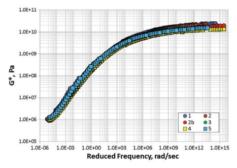
Fig. 5 Master curves of complex modulus, G\*, of the binder recovered from mix samples after one year of service ( $T_{ref} = 25$  °C)—references 1–3 are HyRap sections whereas 4 and 5 are the Control sections
