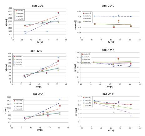
Fig. 3 Results of BBR at -5, -12, -25 °C in function of filler RVs
