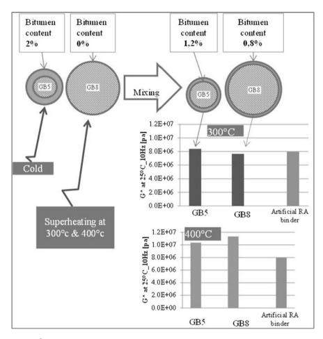
Fig. 3 G\* values of the binder recovered from the GB5 and GB8 glass beads in mixture 1
