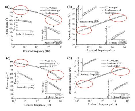
Fig. 4 Master curves at reference temperature of 35 °C. **a** Phase angle master curves for unaged samples. **b** Dynamic modulus master curves for unaged samples. **c** Phase angle master curves for short-term aged samples. **d** Dynamic modulus master curves for short-term aged samples
