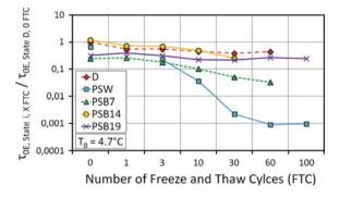
**Fig. 8** Relationship between the relaxation time established at T<sub>0</sub> of 4.7 °C for a specific saturation state "i" ( $\tau_{0E,state \ i,X}$  FTC), expressed in reference to the relaxation time obtained for the D sample ( $\tau_{0E,state \ D,0}$  FTC), and the number of FTC
