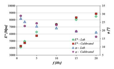
Fig. 2 Calibration for input parameters of Burger's contact model fitted with lab test data
