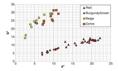
**Fig. 4** b\* versus a\* for the samples accepted by the steering committee. For each colour class the standard is marked in *grey*
