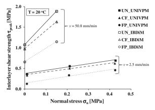
obtained with D = 150 mm and v = 50.8 mm/min, are in reasonable agreement with previous results (Canestrari et al. 2012).
