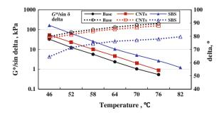
**Fig. 2**  $G^*/\sin\delta$  and phase angle curves from DSR test
