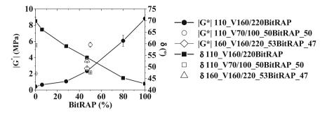
Fig. 2 Complex modulus ( $|G^*|$ ) and phase angle ( $\delta$ ) at 20 °C as a function of BitRAP content for mixtures prepared at 110 and 160 °C
