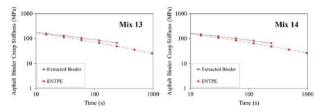
Fig. 6 Back-calculated and extracted creep stiffness of asphalt binder: mix 13 and 14
