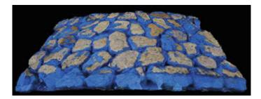
Fig. 6 Painted PSV specimen TIN mesh after painting and accelerated polishing modelled using Zephyr
