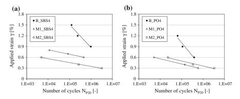
Fig. 4 Comparison between bitumens and mastics fatigue curves in terms of  $N_{P20}$ : a Materials modified with SBS. b Materials modified with PO
