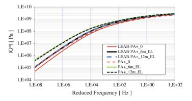
Fig. 4 G\* shear modulus mastercurve comparisons between fresh, 6 and 12 month old mortars from LEAB-PA16+ and standard PA16+ mix at  $T_{ref} = -10$  °C
