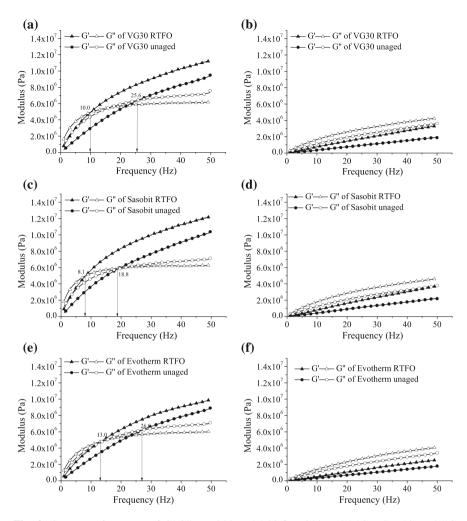
**Fig. 3** Crossover frequency of G'-G" **a** VG30 at 25 °C **b** VG30 at 35 °C **c** Sasobit at 25°C **d** Sasobit at 35 °C **e** Evotherm at 25 °C **f** Evotherm at 35 °C
