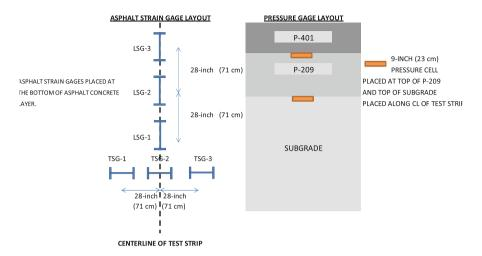
Fig. 3 Pavement instrumentation/sensor layout
