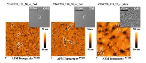
Fig. 3 AFM topography images of the surface of V160/220\_110\_20\_cr\_fast, V160/220\_160\_ 20\_cr\_fast and V160/220\_110\_20\_cr\_slow. OM = optical microscopy images obtained with microscope placed above the head of the AFM instrument. The ellipses show examples of the "bee" structures. Scan area is  $50 \times 50 \ \mu\text{m}^2$
