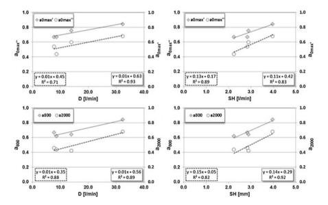
Fig. 6 Drainability and sand height versus a<sub>0max'</sub>, a<sub>0max'</sub>, a<sub>800</sub>, a<sub>2000</sub>
