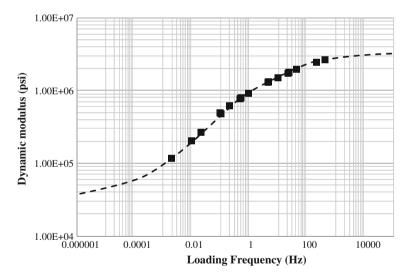
Fig. 5 Dynamic modulus master curve (1 psi = 6.894 kPa)
