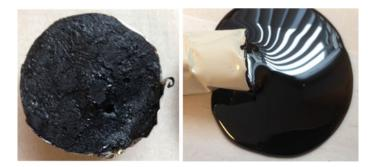
Fig. 6 Photograph of the bottom (*left*) and top (*right*) part of the toothpaste tube, after the storage stability test, B11 + 3 % PPA
