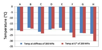
Fig. 10 Comparison between the temperature at 200 MPa complex modulus (at 0.1 rad/s) and the temperature at 300 MPa stiffness
