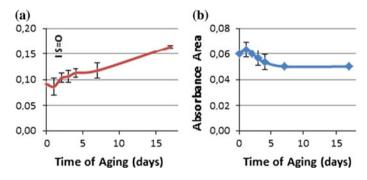
**Fig. 2** a Change in  $I_{S=0}$  0–17 days for bitumen oven aging. **b** Change in  $A_{1600}$  for 0–17 days of bitumen aging (average of three samples)
