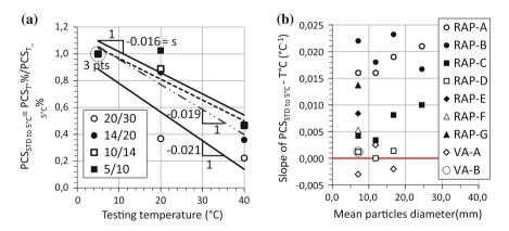
Fig. 7 Representation of the effect of the testing temperature on the potential RAP material fragmentation: **a** example of relationships between the  $PCS_{STDat5^{\circ}C}$  values and the testing temperature of RAP-A; **b** relationship between the rate of change of  $PCS_{STDat5^{\circ}C}$  with temperature and the mean size of all tested RAP particles
