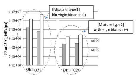
Fig. 5 Summary and comparison of the DSR results obtained on the bitumen from the GB5 and GB8 glass beads as used in mixtures 1 and 2
