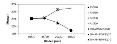
Fig. 5 Evolution of R&BT after artificial ageing RTFOT and PAV
