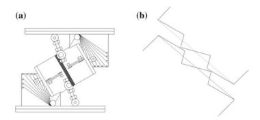
Fig. 3 Schematic drawing of the SISTM (a) and representation of the dilatancy behavior (b)
