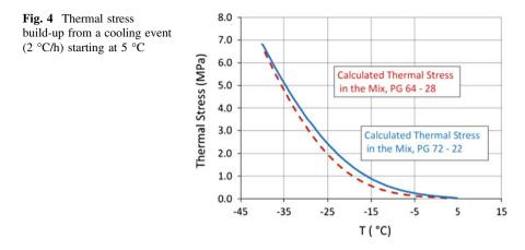
The 4-mm DSR/ABCD method provides estimation of the necessary input for the MEPDG thermal cracking model, i.e. the mix thermal stress development from the 4-mm DSR test and mix tensile strength estimated from the ABCD test. Both tests are relatively simple and rapid, which is an important consideration given that the asphalt mixture testing in accordance with AASHTO 322-07 is expensive and time-consuming.
