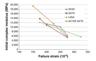
Fig. 6 Initial complex modulus versus failure strain
