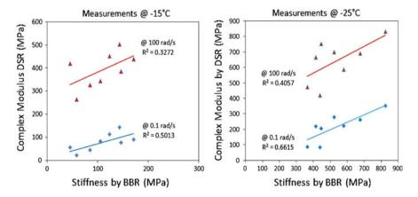
Fig. 6 Correlation between complex modulus by 4-mm DSR and stiffness by BBR
