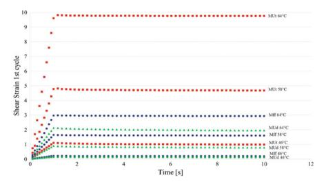
Fig. 3 Strain/time for the first cycle of RCR test at 1 kPa at 46, 58 and 64 °C
