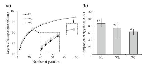
Fig. 4 Mixture compactability: a SGC compaction curves, b compaction energy index (CEI)
