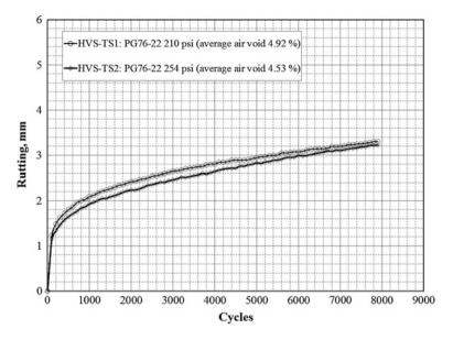
Fig. 6 APA test results on cores extracted from HVS-A test strips
