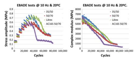
Fig. 5 Stress amplitude and complex modulus versus the number of cycles in the EBADE tests
