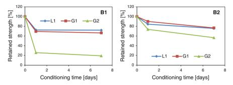
Fig. 8 Effect of moisture conditioning time on tensile strength of different aggregate-bitumen combinations. In general acidic aggregate performed worse than basic aggregates. The combination of bitumen B1 with aggregate G2 performed worst
