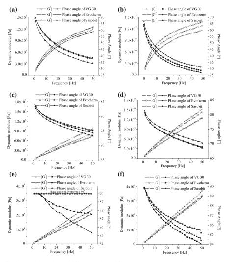
**Fig. 2** Dynamic modulus of different samples at different temperatures. **a** Unaged samples at 25 °C. **b** RTFO aged samples at 25 °C. **c** Unaged samples at 45 °C. **d** RTFO aged samples at 45 °C. **e** Unaged samples at 75 °C. **f** RTFO aged samples at 75 °C
