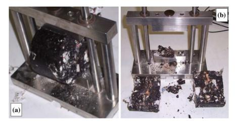
Fig. 3 Type of fatigue failure: a Ductile. b Fragile
