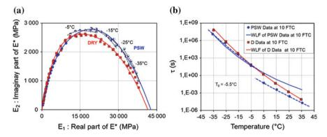
Fig. 6  $E^*$  results obtained for the first 10 FTC of the PSW and D samples: a cole-cole plane, b relationship between the relaxation time and the  $E^*$  testing temperatures
