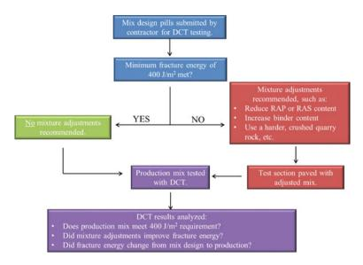
Fig. 3 Flowchart of mixture testing and adjustment process
