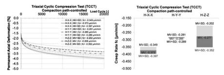
Fig. 4 TCCT results for path-controlled compaction: creep curve (*left*), and creep rate (*right*)
