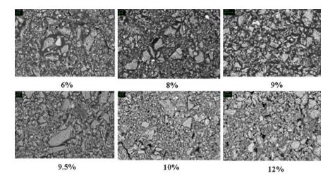
Fig. 5 Images at different percentages of filler content (by weight of the aggregates excluding the filler) for brick dust as filler
