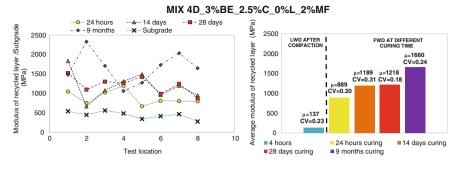
Fig. 4 Performance over time: mixture 4D
