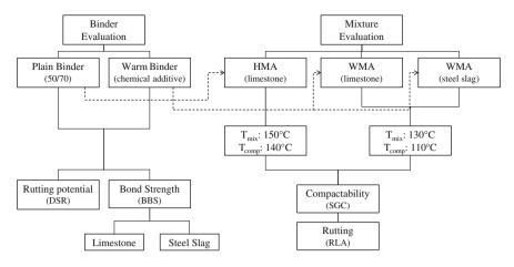
Fig. 1 Experimental plan
