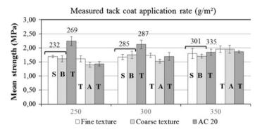
Fig. 3 Results of interlayer bonding tests (SBS, TAT)-Impact of tack coat application rate and nature and preparation of the underlayer for the interface between SMA 10 and three underlayers. Note that the measured tack coat rates are indicated above each bar. The *error bars* represent the standard deviation
