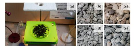
Fig. 1 a Set for digital picturing of tested samples; b Porphyry; c Limestone; d Basalt; e Blast furnace slag samples
