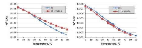
Fig. 2 G\* (at 1 Hz) versus temperature before and after adding PPA, B2 (left), B11 (right)
