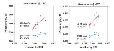
Fig. 9 Comparison between phase angle by 4-mm DSR and m-value by BBR
