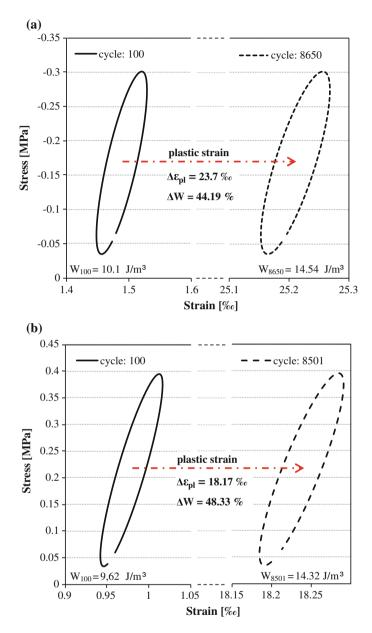
Fig. 7 Hysteresis loops at cycle 100 and at failure (cycle  $N_{Macro}$ ) for indirect tensile test (**a**) and uniaxial tension test (**b**)
