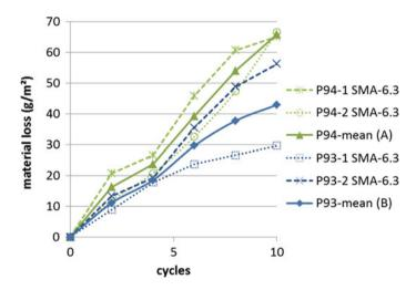
Fig. 5 Test results for SMA 6 (mix A and B, with different grading), at 40 °C
