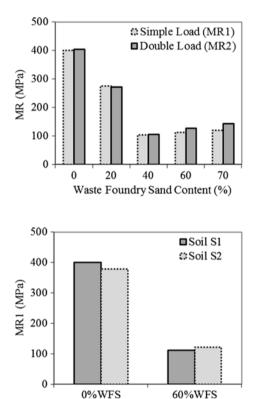
**Fig. 9** Average MR values of soil-sand mixtures using control materials in a low volume traffic road structure, for simple load
