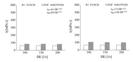
Fig. 5 Viscosity (n) versus shear rate (SR) of B1-NCB blends
