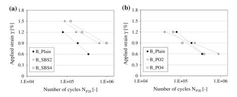
Fig. 2 Fatigue curves in terms of  $N_{P20}$  for all bitumens: **a** Plain and PMBs with SBS. **b** Plain and PMBs with PO
