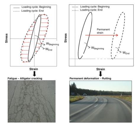
Fig. 5 Interpretation of a fatigue test (*left*) and a permanent deformation test (*right*); hysteresis loops for the loading cycles at the beginning and at the end of the test (cf. Di Benedetto 2013)
