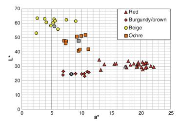
Fig. 5 L\* versus a\* for the samples accepted by the steering committee. For each colour class the standard is marked in grey
