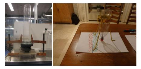
Fig. 6 Illustration of permeability lab test (*left*) and Breda bottle test (*right*), *green* is old PA, *red* is new PA
