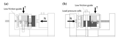
Fig. 4 SDSTM in the two test configurations: inhibited (a) and allowed dilatancy (b)
