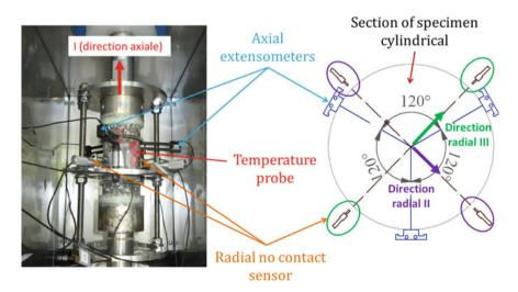
Fig. 1 Left general view of the experiment developed at ENTPE to measure the axial strain and the radial strain. Right section of the cylindrical specimen and strain measurement devices
