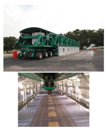
Fig. 1 FAA's heavy vehicle simulator-airfields mark VI (HVS-A)
