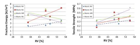
Fig. 6 Influence of filler fractional voids on mastics tensile limits
