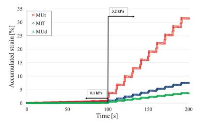
Fig. 6 MSCR test results at @ 46 °C
