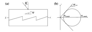
Fig. 2 Bolton's saw blades model (a) and identification of  $\Phi'_{crit}$  on the Mohr circle of stress (b)
