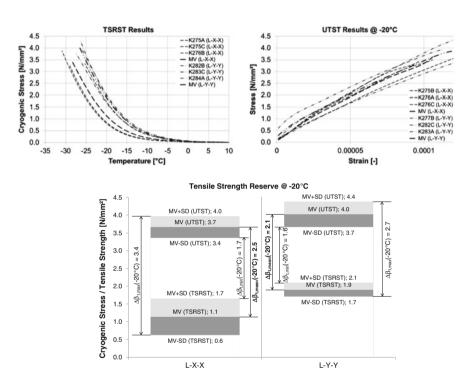
Fig. 2 TSRST results (upper left), UTST results (upper right) and tensile strength reserve (below)
