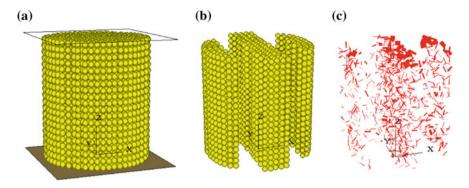
Fig. 3 Discrete element model in  $PFC^{3D}$ . a DEM model. b Slices of the model. c Tensile forces in slice model
