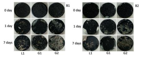
**Fig. 9** Failure surface of aggregate-bitumen bonds exposed to moisture: top bitumen B1; bottom bitumen B2. The effect of bitumen type is minimal compared with the effect of aggregate type
