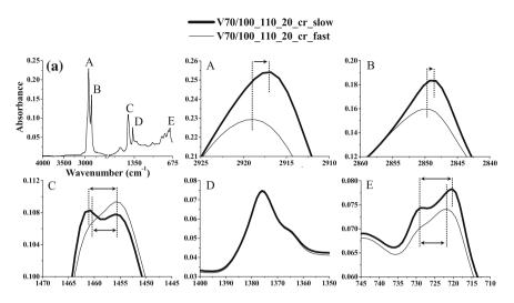
**Fig. 5** ATR-FTIR spectra for V70/100\_110\_20\_cr\_fast and cr\_slow. **a** V70/100\_110\_20\_cr\_fast full spectrum. *A*, *B*, *C*, *D* and *E* show close-ups at  $\sim$  2920,  $\sim$  2850, 1460–1455,  $\sim$  1375 and 730–720 cm<sup>-1</sup>, respectively. The *dotted lines* and the *arrows* show shifts and splitting of the peaks
