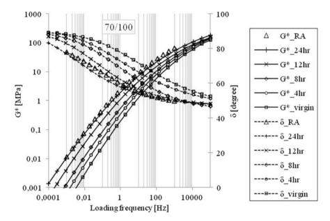
Fig. 2  $~G^*$  and  $\delta$  master curves of the virgin 70/10 and 70/100 pen bitumen aged for several hours using the RCAT at 25  $^{\circ}C$
