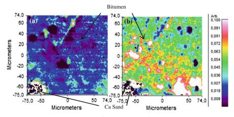
Fig. 3 FTIR-ATR microscope  $1030 \text{ cm}^{-1}/(1460 + 1376 \text{ cm}^{-1})$  band ratio images for: **a** unaged mastic and **b** mastic aged for 14 days in oven (*right*)
