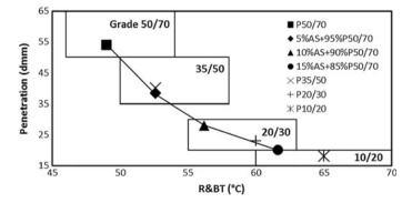
Fig. 3 Properties of asphaltite modified bitumens
