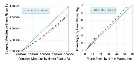
Fig. 3 Comparison between 4 and 8 mm plates (sample B)
