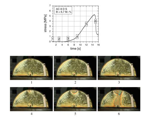
Fig. 6 Visualization of the deformation evolution during a monotonic bending test (AC 8 D S)
