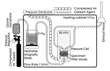
Fig. 1 Aging setup for VAPro
