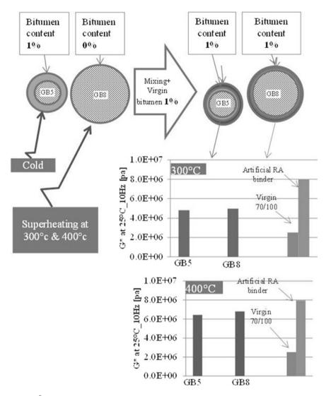
Fig. 4 G<sup>\*</sup> values of the binder recovered from the GB5 and GB8 glass beads in mixture 2
