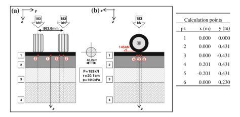
Fig. 4 Pavement model with B737-800 loads: a y-z view, b x-z view and calculation points
