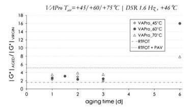
Fig. 5 Change in dynamic shear modulus  $|G^*|$  of bitumen recovered from lab-aged HMA specimen to virgin bitumen sample
