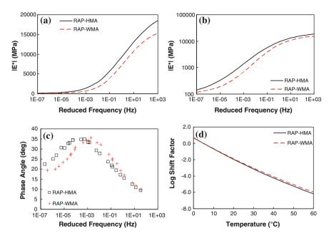
Fig. 1 Linear viscoelastic characterization for RAP-HMA and RAP-WMA mixtures: **a** dynamic modulus mastercurve in semi-log space, **b** dynamic modulus mastercurve in log-log space, **c** phase angle mastercurve, and **d** time-temperature shift factor function
