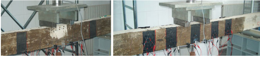
Fig. 6.24 Possible shear U-shaped anchoring devices (Ceroni 2010)
