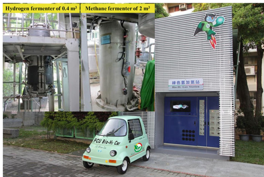
Fig. 2.2 Two-stage biohydrogen and biomethane production pilot plant in Feng Chia University campus with hydrogen fermenter of 0.4 \text{ m}^3 and methane fermenter of 2 \text{ m}^3
