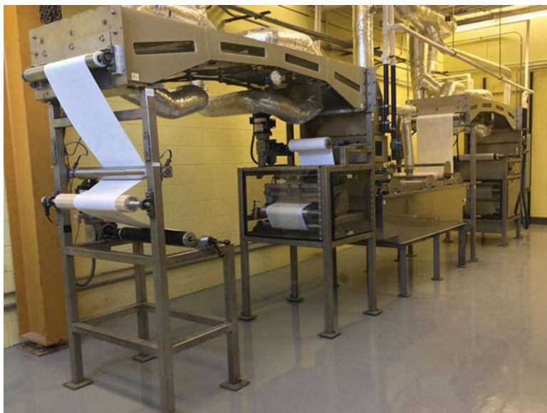
Fig. 11.6 Pilot-scale membrane coating machine consisting of the coating section, rinse tank, and thin-film-casting (TFC) assembly
