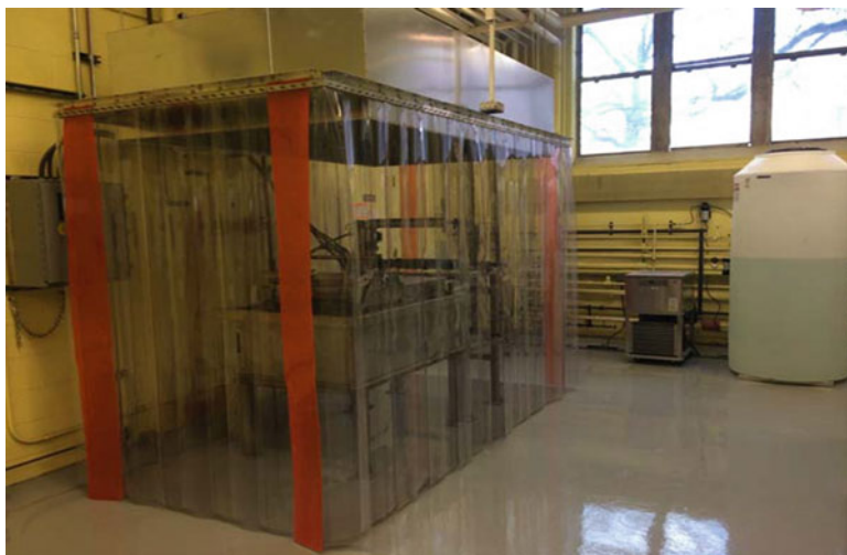
Fig. 11.7 Pilot-scale membrane casting machine for fabricating nanoporous membranes using the phase inversion process
