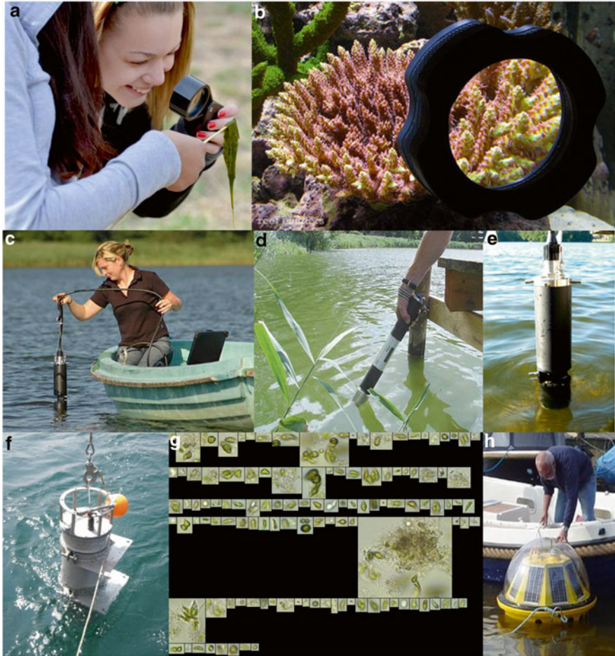
Fig. 1 Studying algae in the field (a, b) Magnifying glass, (c) Portable spectrometer, (d) AlgaeTorch, a field instrument used to measure chlorophyll directly in the water body, from live algae (e) FluoroProbe, a multiwavelength field fluorometer (f) FlowCytobot, an in-situ automated submersible imaging flow cytometer (g) Images of algae obtained through FlowCam, an imaging cytometer (h) CytoBuoy, a real time monitoring flow cytometer
