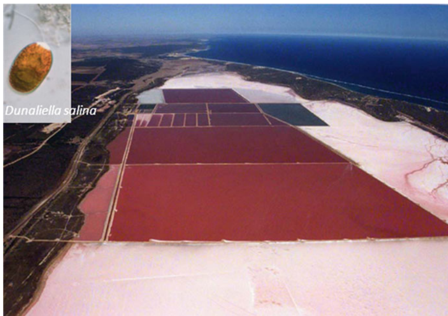
Fig. 17 Dunaliella salina production plant in Australia (operated by Cognis Nutrition & Health at Hutt Lagoon), it is the largest production plant of algae in the world
