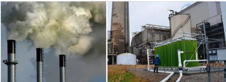
Fig. 19 Carbon reduction technology-Flue gas from the CO 2 emission plant provides carbon dioxide to feed algae in fuel tanks
