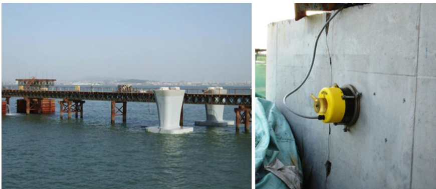
Fig. 8.40 Testing Qingdao Bay Bridge with PERMIT by Tsinghua University
