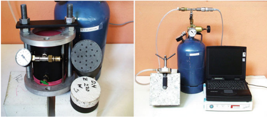
Fig. 4.8 Test setup for evaluation of permeability exponent [19]
