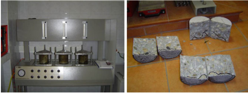
Fig. 4.16 Water permeability testing in the laboratory
