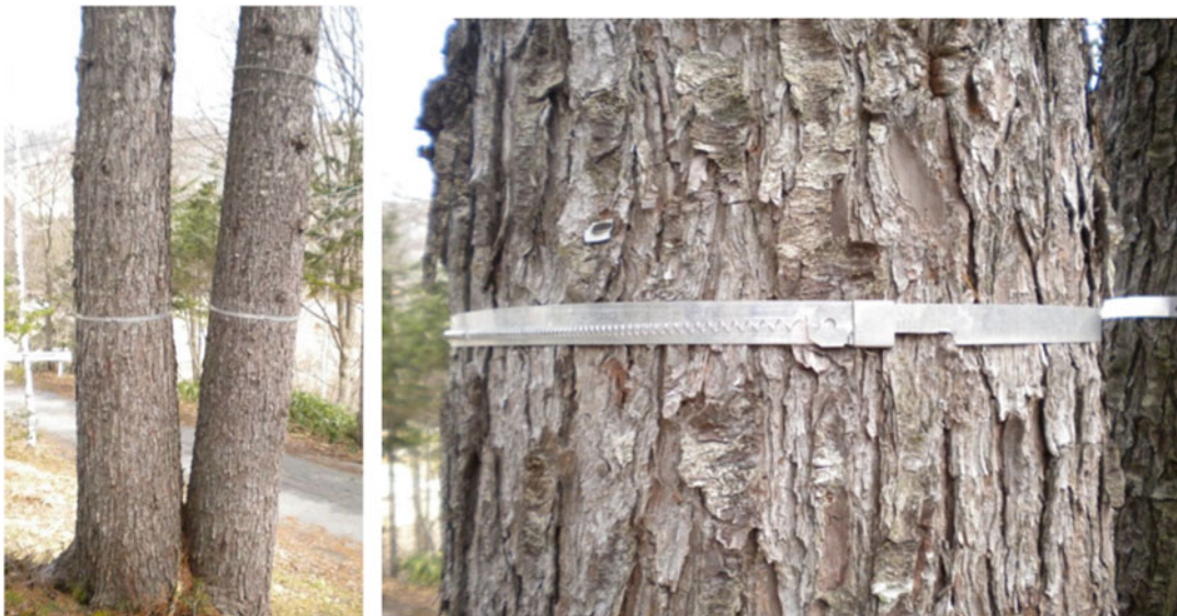
Fig. 12.4. Example of a dendrometer used to measure annual tree growth under field conditions. This dendrometer consists of an aluminum band with a stainless spring
