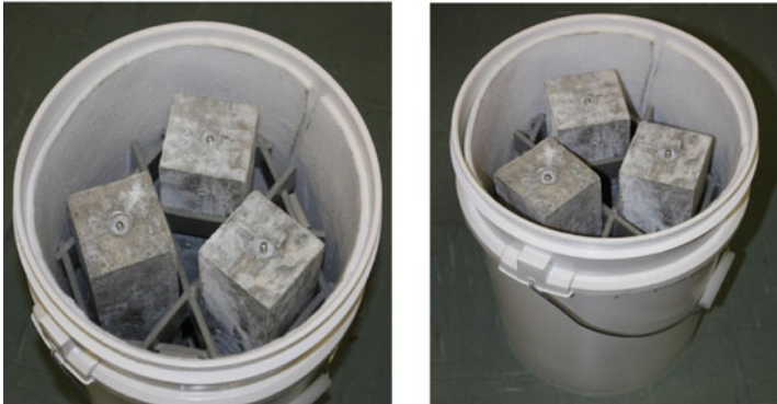
Fig. A.1 Concrete prism specimens in the storage container
