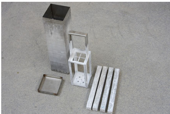
Fig. 1 One suitable container, showing the internal framework for holding the mortar-bars (note the perforations in the base, to accommodate the measuring studs)
