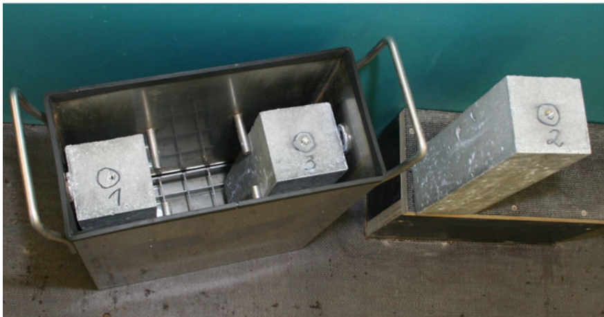
Fig. 2 Sealable containers for storing concrete prisms (dimensions in mm)
