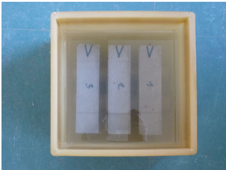
Fig. 3 Container with set of 40/40/160 mm bars submerged in NaOH-solution
