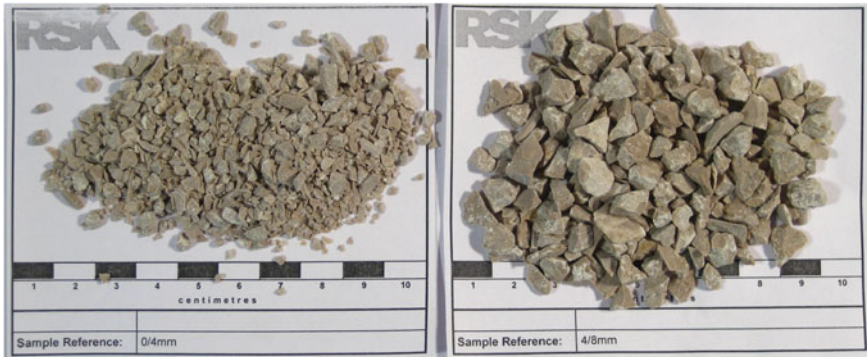
Fig. 2 Comparison of AAR-2 ( left ) and AAR-5 ( right ) aggregates
