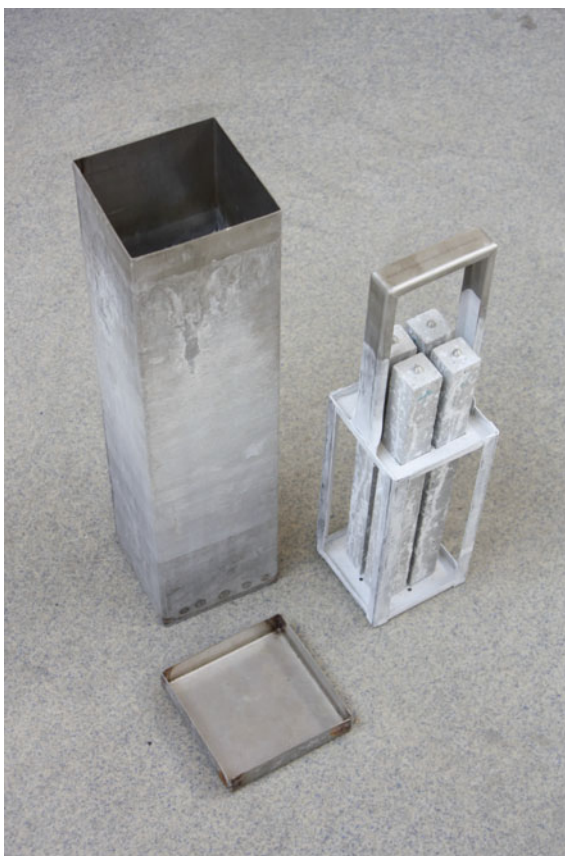
Fig. 2 As Fig. 1, but showing the set of mortar-bars held in the internal framework
