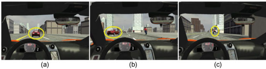
Fig. 2.3 Stimuli related to emergencies (a) Sharp braking by the leading vehicle's brake light, (b) Sharp braking by cutting-in, (c) Sharp braking by a pedestrian
