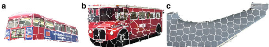
Fig. 8.3 Entropy gain (Sect. 8.3.2): When segments a and b are merged, the increase of entropy is not as big as if they were merged with c . Homogeneity criterion (Sect. 8.3.3.1): Segment c is homogeneous. It presents smooth variation due to shading and lighting. Segments a and b are not homogeneous. Both entropy and homogeneity are calculated from the small (first level \mathcal{D}_i^1 ) segments, illustrated with white contours
