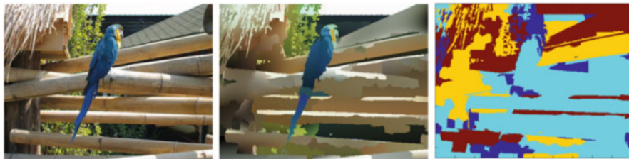
Fig. 8.6 Different segments can have different polynomial order k . Left : original. Center : polynomial base approximation. Right : order of the polynomial, where: dark-blue : k = 0 , light-blue : k = 1 , yellow : k = 2 ; red : k = 3
