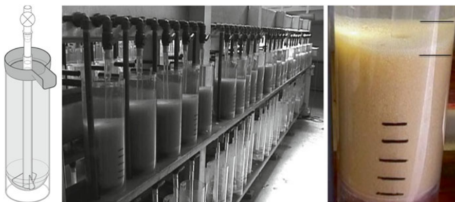
Fig. 11.3 Incubation jar (line drawing), a double row lineup of jars with incubating Walleye eggs, and a close-up of jar showing layer (double bar) of dead eggs that will be removed with siphon
