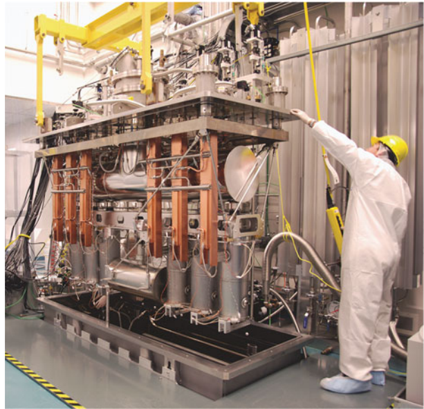
Fig. 12 Cryomodule SCC1 assembly prior to the first cold test
