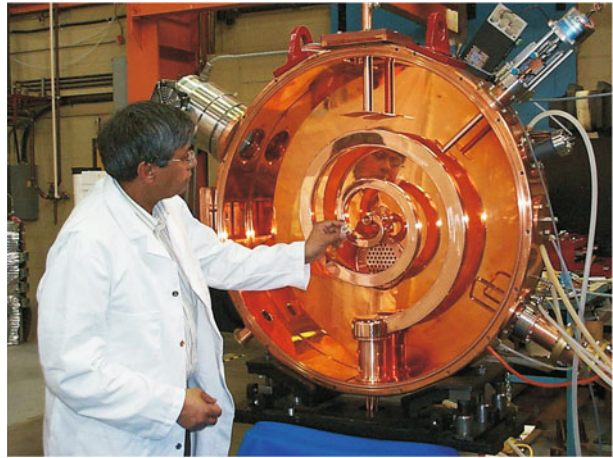
Fig. 4 MEBT 35 MHz rebuncher to match the beam into the ISAC-I DTL
