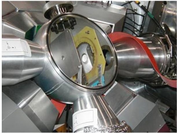
Fig. 6 BAMBINO facility installed at TIGRESS, with the side access panel of the scattering chamber removed, showing one S3 detector mounted downstream of the target location with a blank collimator plate in place of an upstream detector
