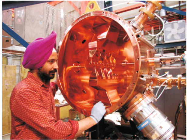
Fig. 8 DTL Tank 1 structure
