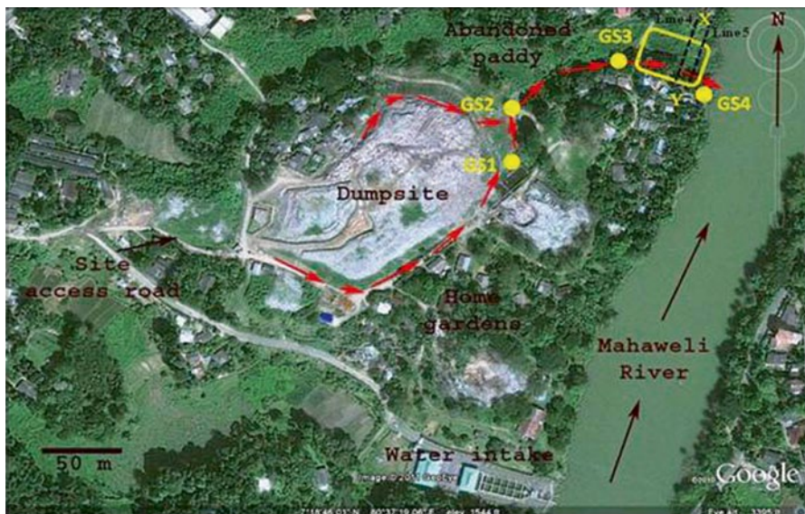
Fig. 11.3 Schematic diagram of the leachate drainage channel (red arrows), leachate sampling points (yellow dots), resistivity survey area (yellow rectangle), and 2D profile lines 4 and 5 with direction X-Y (black dotted line) at the Gohagoda dump site
