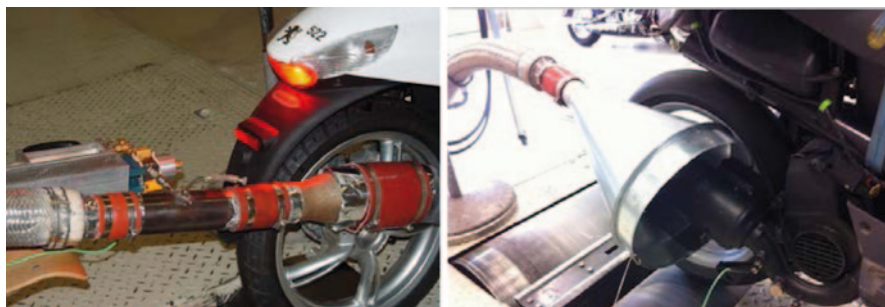
Fig. 1 Minidiluter. Passage of exhaust gas from tailpipe to CVS: closed ( left ), open ( right )
