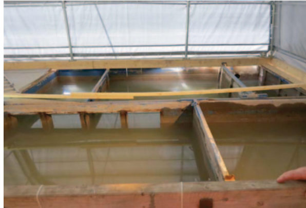
Fig. 2 Example of sedimentation pool constructed to enable minimal water turbulence and S-shaped flow
