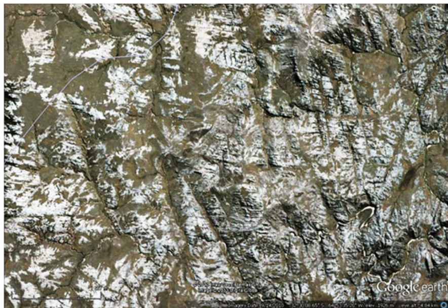
Fig. 10 Google Earth image showing the characteristic drainage network in granitic environments
