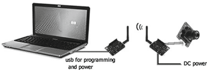
Fig. 1 Wirelessly paired microcontrollers with a camera module attached
