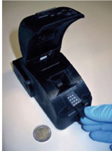
Fig. 5 The NeoMark RT-PCR tool (Source: NeoMark). The NeoMark RT-PCR tool is a portable, real-time, low-cost RT-PCR that can work as an alternative to microarrays for examining patient's RNA extracted from tumor specimens and/or lymphocytes. The device is composed of a core silicon chip containing heaters and thermal sensors, a cooling fan, and an optical system that detects the fluorescence intensity of the monitored reaction. Reused with permission from STMicroelectronics
