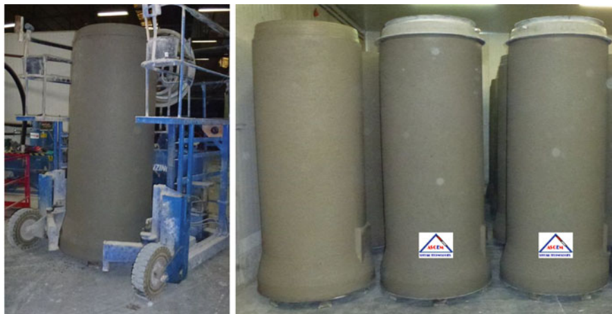
Fig. 11.13 Production of pipes
