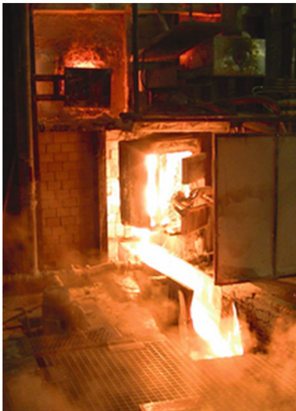
Fig. 11.10 Outflow of the glass melt into the cooling unit
