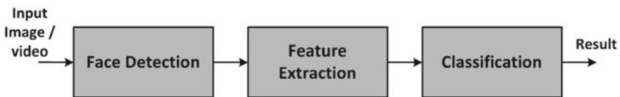
Fig. 1 Block diagram of a generic face recognition system
