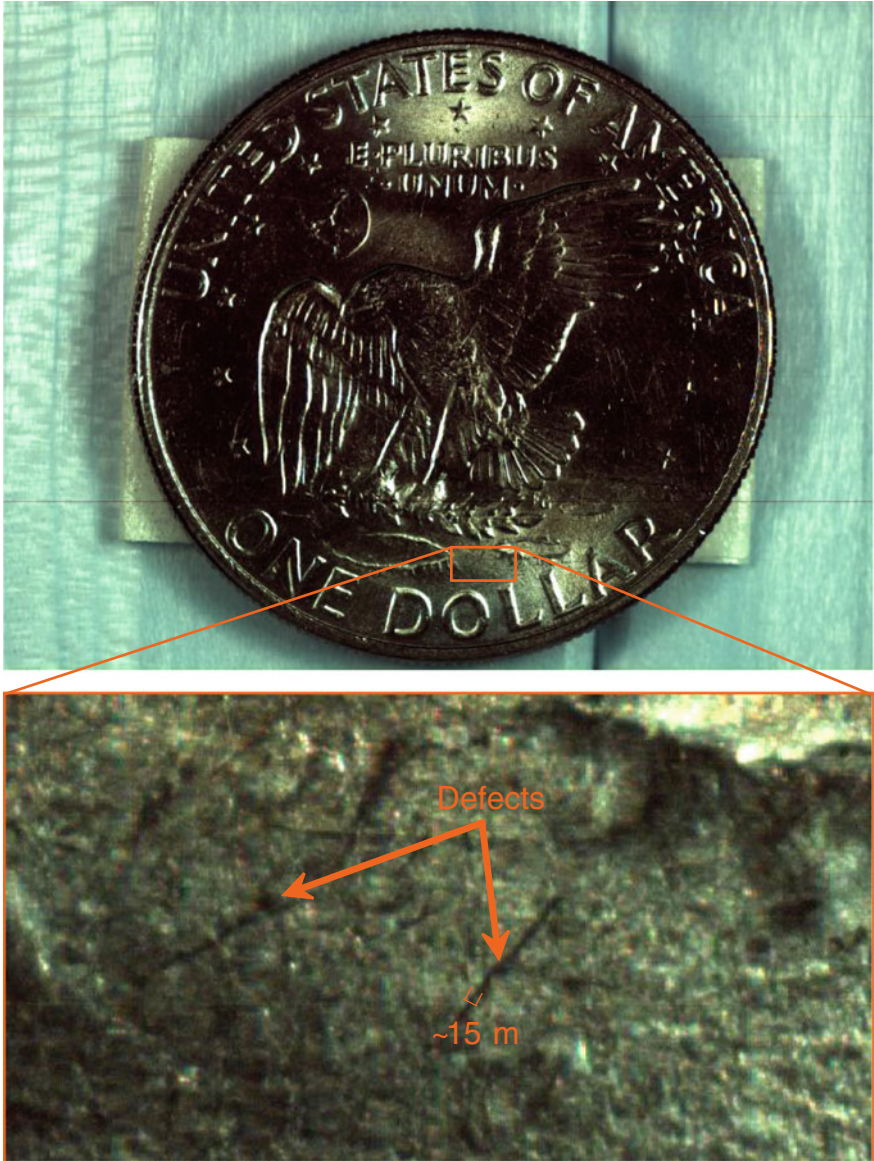
Fig. 20 Close-range multi-line CCD image of the tail of a silver dollar, color misalignment has been corrected. The resolution of the image is 6k \times 8k pixels
