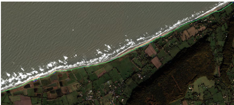
Fig. 19 Coastline extraction on Normandy coast from a QuickBird image (©Digitalglobe), extracted coastline in green and reference coastline in blue (results are dilated for better visualization) [39]
