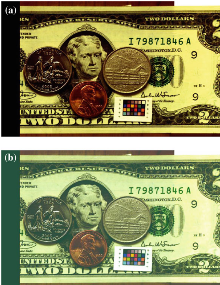
Fig. 21 Close-range multi-line CCD image of a two-dollar bill and several coins. a Before color calibration. b After color calibration. The resolution of the image is 6k \times 10k pixels
