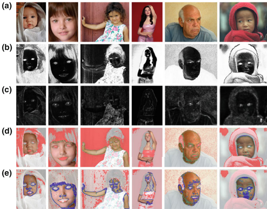
Fig. 10 Skin detection results obtained using the SPM color filter and refined using the Gabor wavelets: original image (a), skin probability map (b), texture image (c), segmentation using the threshold \Theta = 180 (d), image after applying the texture mask for various \Theta_T ( 20 \leq \Theta_T \leq 120 ) (e)
