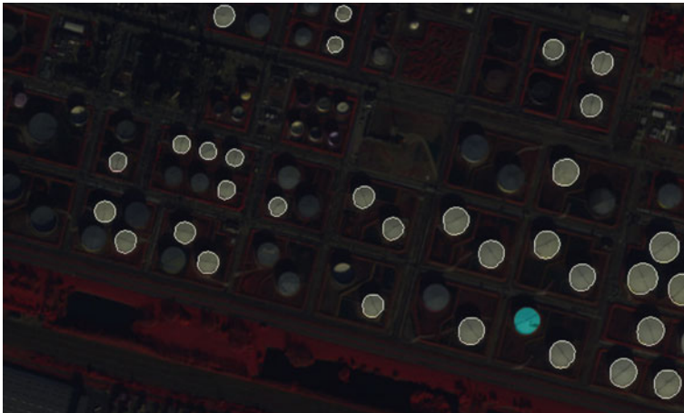
Fig. 21 Petroleum tank extraction on Le Havre harbor QuickBird image(©Digitalglobe) [39]. Correct detections are surrounded by white boundary, false negative are given in cyan (there is no false positive)
