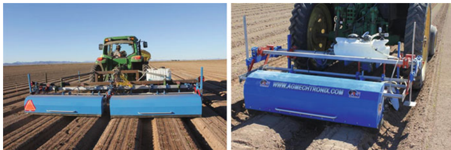
Fig. 6.17 Row crop thinner (Source: http://www.agmechtronix.com/RCT.aspx )
