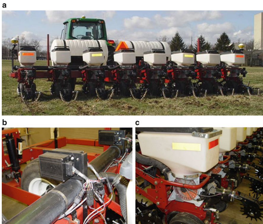
Fig. 6.12 Final prototype planter with GPS for generation of differential toolbar speed (a). Single row CAN node and motor controller (b). DC gear motor drive with sensor integration (c)
