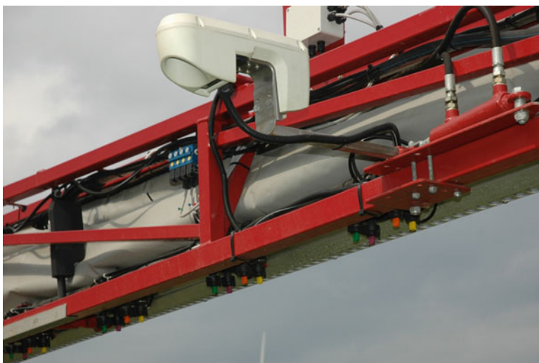
Fig. 10.3 Detail of the SensiSpray spraying system. The GreenSeeker sensor is used to determine the amount of biomass, and the spray volume is adjusted by switching on and off one to four nozzles in the nozzle holder
