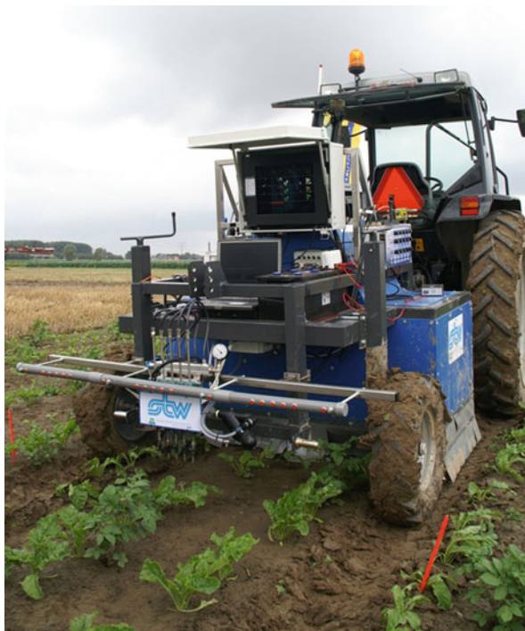
Fig. 10.4 Weed control system for control of volunteer potatoes within rows of sugar beets. Two cameras are mounted under the hood and the volunteer potatoes are micro-sprayed with the spray unit in the rear
