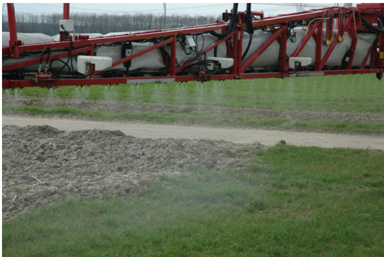
Fig. 10.2 SensiSpray system mounted on a sprayer with air support to prevent drift
