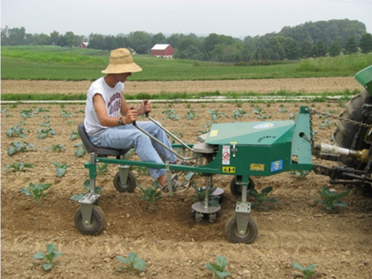
Fig. 7.5 ECO weeder requires an operator to move rotating weeding mechanisms with tines (HCC 2011)
