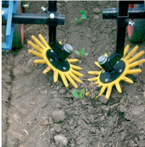
Fig. 7.2 Finger weeder uses rubber spikes that are pointed at an angle towards the crop (Weide et al. 2008)
