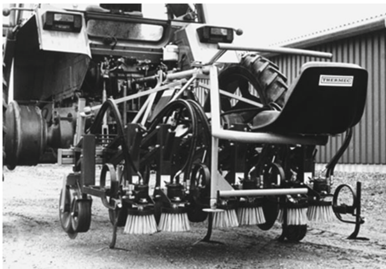
Fig. 7.4 Vertical-rotating brush weeder uses hydraulics and requires an operator (Melander 1997)
