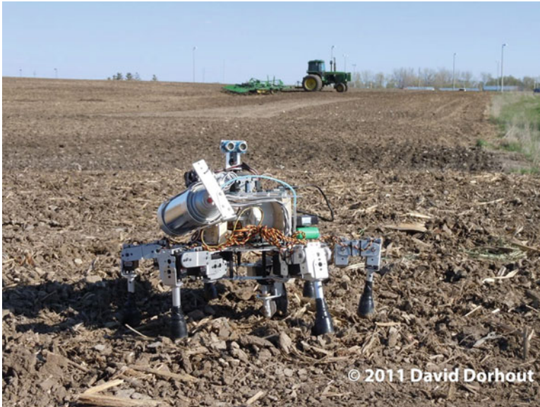
Fig. 15.5 Prospero, the robot that plants and manages crops fields of the future (Reprinted with permission from Dorhout R&D LLC (LLC ( http://dorhoutrd.com )))
