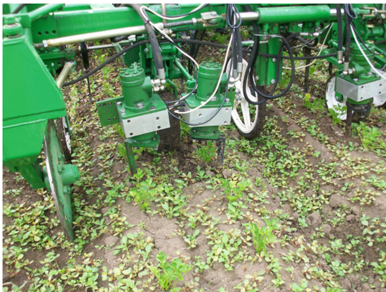
Fig. 9.2 Intra-row weeding in celery with the Robocrop InRow cultivator (From Fennimore et al. in press )
