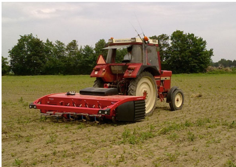
Fig. 10.1 Steketee mechanical intrarow weed control system. Cameras detect the plants and the weeds are controlled by pneumatically guided hoes
