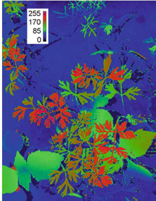
Fig. 5.9 Pseudocolor 3D depth image adapted from Piron et al. (2009). Higher valued pixels ( red and orange colors ) are closer to the camera than lower valued pixels ( green and blue colors ). The 3D method illustrates the potential value in 3D image methods for dealing with overlapped foliage, which typically causes leaf shape recognition problems in a 2D top view of the scene
