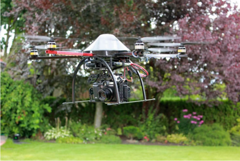
Fig. 5.1 Photograph of a miniature UAV helicopter equipped with a consumer grade digital color camera and GPS navigation system for low-altitude aerial imaging (Mikrokopter 2012. Reprinted with permission from http://www.mikrokoetter.de )
