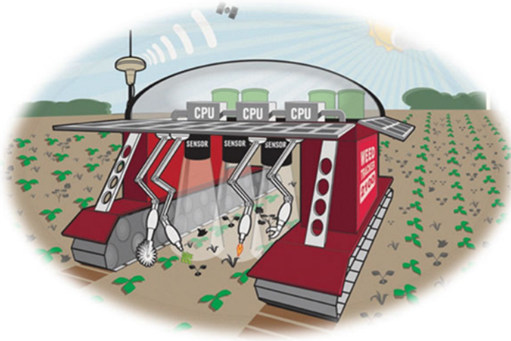
Fig. 15.2 Weed robots of the future will have all of the control tools and a decision support system on a single platform that moves autonomously through the field. Not only that, but also UASs will circle overhead and work directly with on-the-ground robots through wireless communications (Drawing courtesy of S.L. Young)
