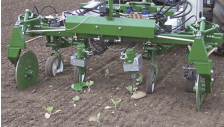
Fig. 7.6 Automated weeder machine uses hydraulics to rotate semi-circle discs (Tillett et al. 2008)
