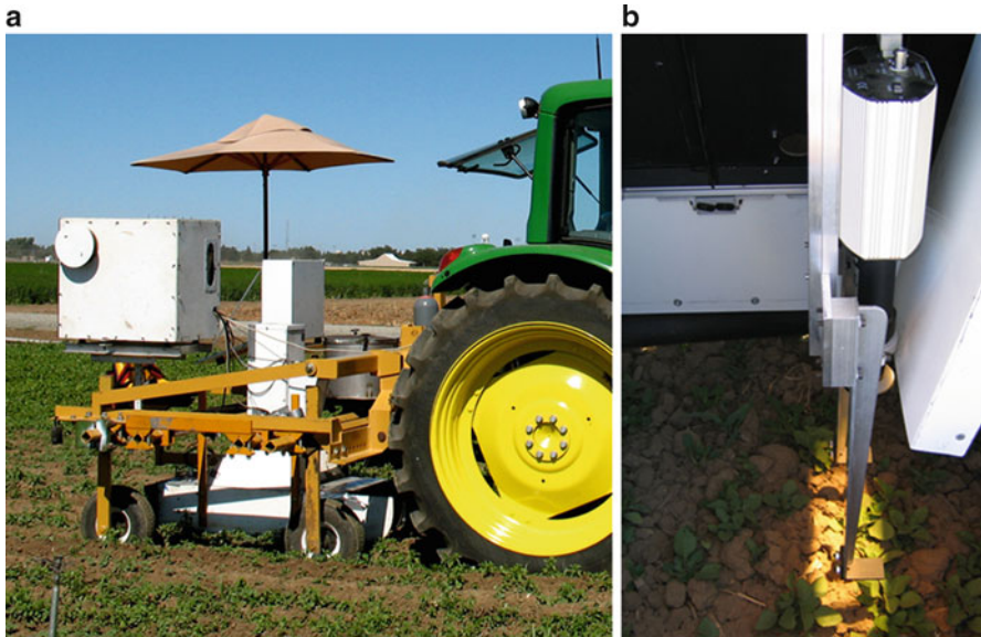
Fig. 5.7 Ground-based hyperspectral imaging system setup for controlled illumination of crop and weed seedlings. (a) Photograph showing the tractor-mounted metal illumination control chamber in the center of the picture. (b) Interior view of the enclosure showing the hyperspectral camera and the illumination system
