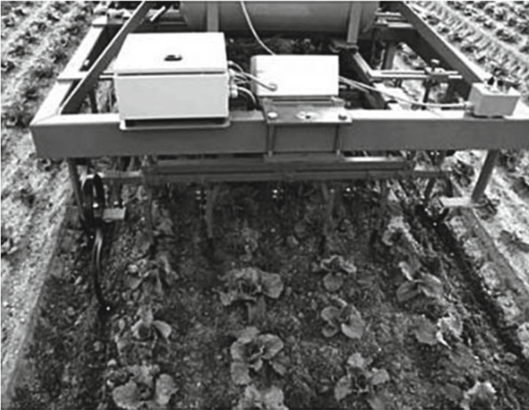
Fig. 7.8 Sarl Radis intelligent weeder from France moves in and out of the crop row (Cloutier et al. 2007)
