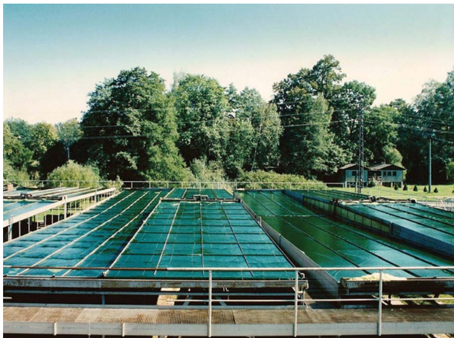
Fig. 3 Open thin-layer photobioreactor of 700 m 2 culture area in Třeboň's Institute. The photobioreactor serves for both growth experiments and production of high-quality biomass used in human and animal nutrition. (Photograph by J. Doucha)
