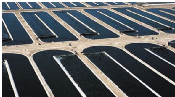
Fig. 11.6 Raceway ponds for growing Spirulina ; courtesy of Robert Henrikson; from Earth Food Spirulina . (Henrikson 2009)
