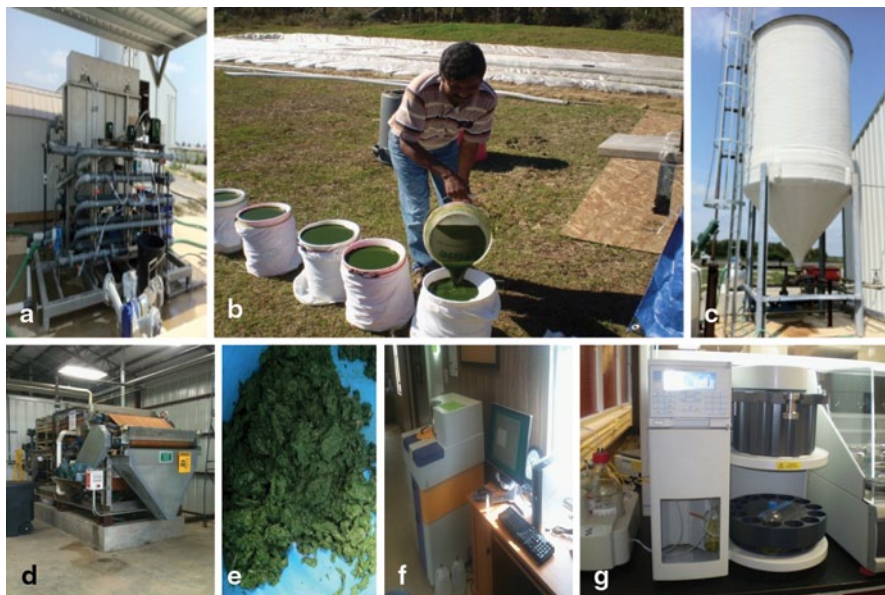
Fig. 4 a DAF unit. b Algal slurry collection. c Holding tank. d Belt press. e Scrapped algae. f Nutrient analyzer. g Extractor
