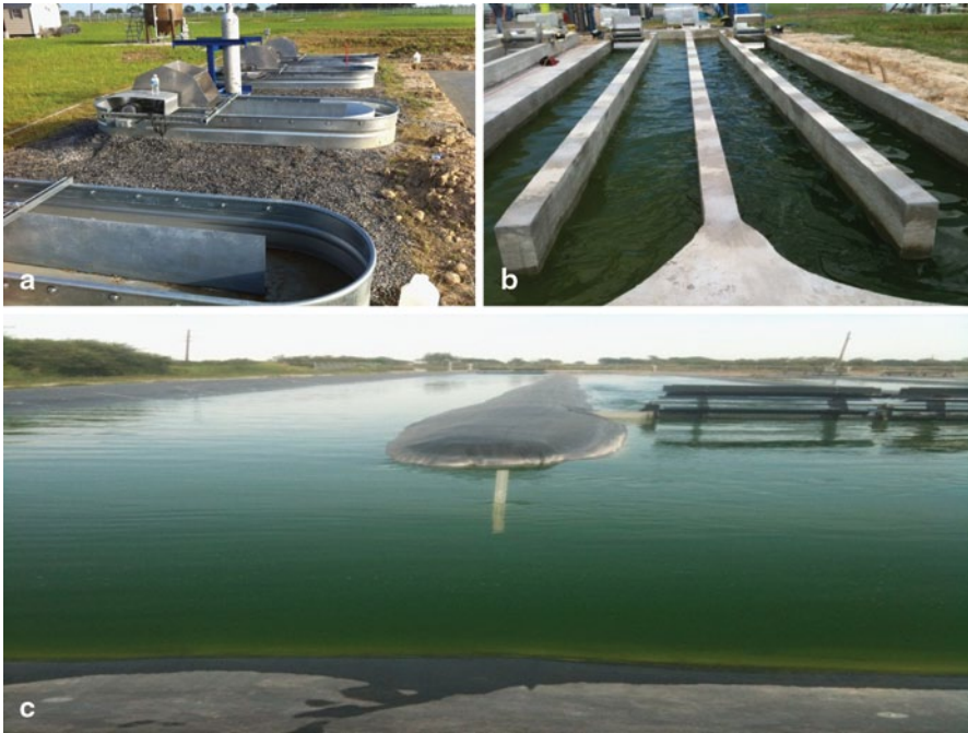
Fig. 1 Open raceway ponds a 3 \times 1 , b 15 \times 1.6 , c 122 \times 14 m (Aquatic Energy LLC)
