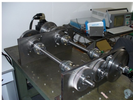
Fig. 1 Conventional cam mechanism stand (grooved radial cam with rocker, constant transfer)
