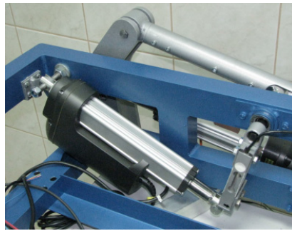
Fig. 4 Lifting drive with measuring beam
