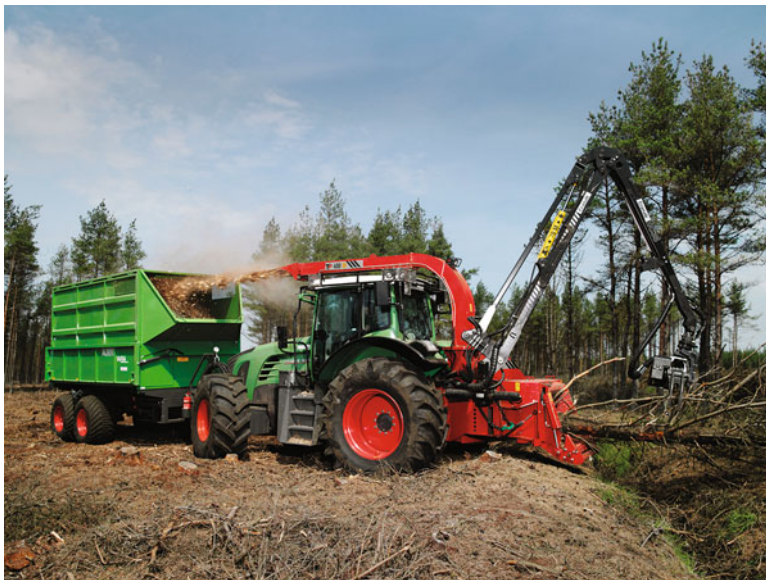
Fig. 6.5 In-field operation using terrain going chipper which feeds directly into a high tipping bin (Photo: Linddana AS)
