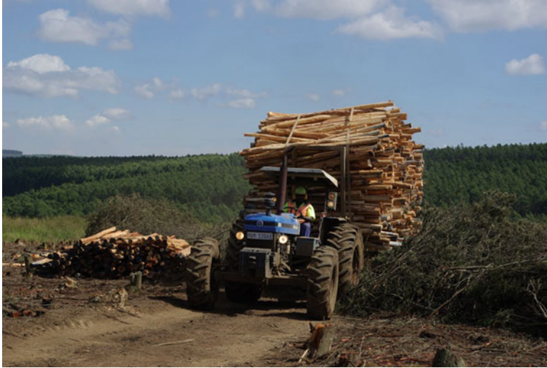
Fig. 6.4 Extraction of a large load of black wattle ( Acacia mearnsii ) using an agricultural tractor and tipping trailer (Photo: Talbot)
