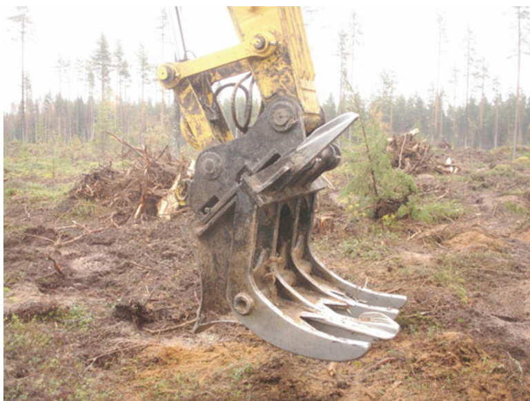
Fig. 6.7 Stump lifting device with splitting knife (Photo: Dahlin)
