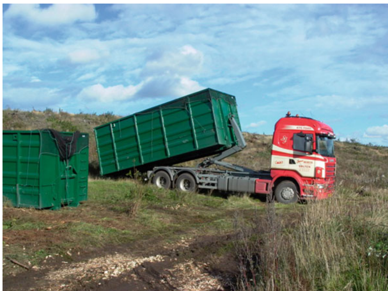
Fig. 6.11 Container truck exchanging chip containers at landing (Photo: Talbot)
