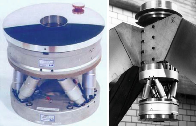
Fig. 6.2 Secondary system attached to top-end structure and vanes (in lab at MPIA, Heidelberg). Note constrained-layer viscous damping panels on the vane sides!
