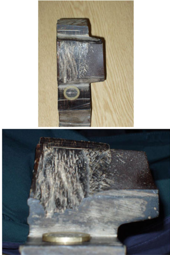
Fig. 2 Oilfield pipeline fibreglass diffuser section after cavitation erosion damage [plan view ( top ) and elevation ( bottom ), scale indicated by €1 coin]
