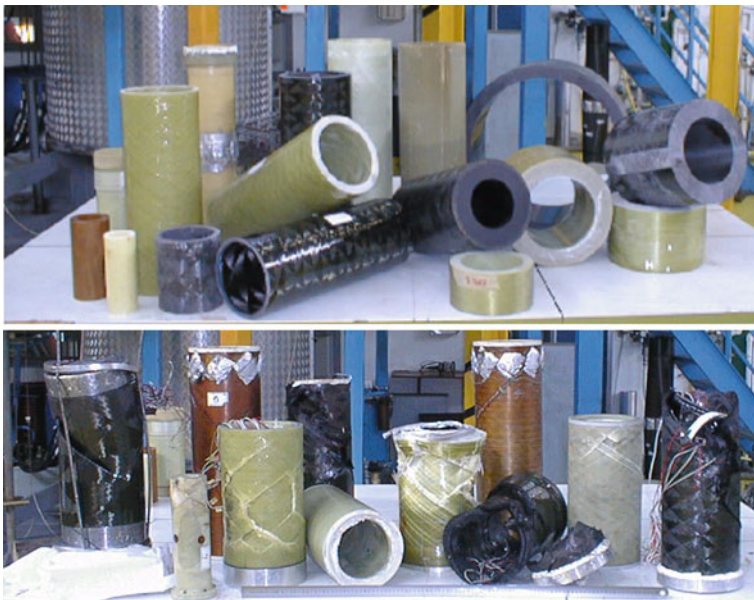
Fig. 4 Deep sea cylinders before and after hydrostatic compression testing
