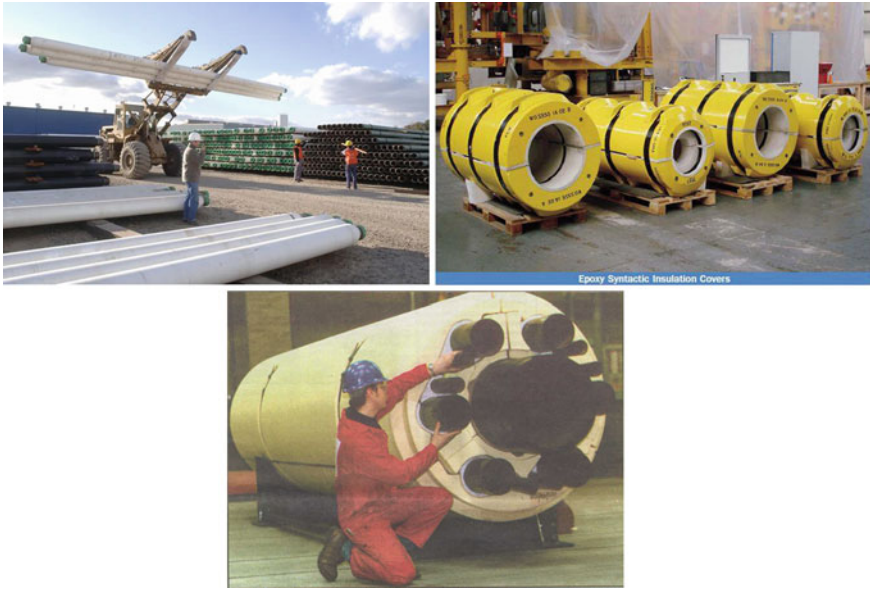
Fig. 9 Syntactic foam materials for deep sea oil and gas applications (pipe, buoyancy module, riser tower)
