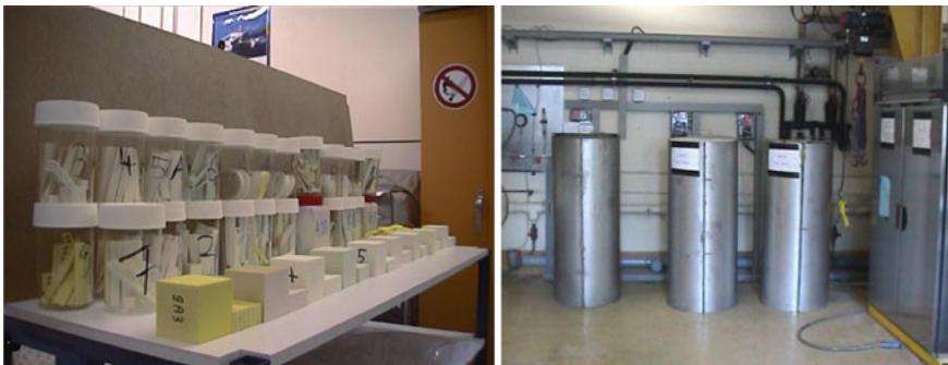
Fig. 10 Syntactic foam materials samples and aging test equipment enabling simultaneous application of pressure, temperature and sea water immersion
