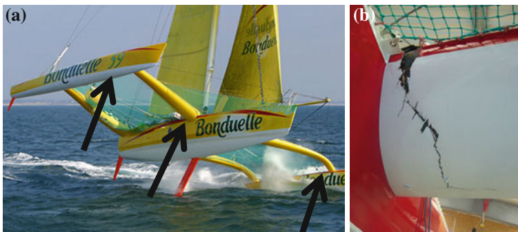
Fig. 14 a Areas exposed to wave impacts. b Example of damage area due to wave impacts
