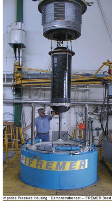
Composite Pressure Housing * Demonstrator test – IFREMER Brest.
