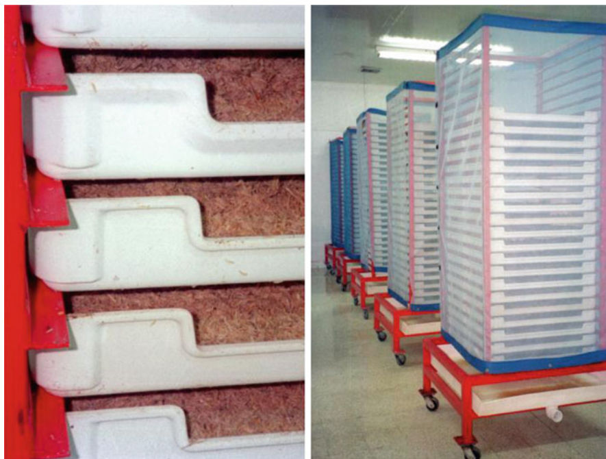
Fig. 15.5 Mass-rearing medflies Medfly larvae are reared in large diet-filled trays that are stacked on carts or trolleys ( on right ) and held in large environmentally controlled rooms. Mature larvae migrate from the diet (some are visible on the sides of trays at left ) and, in most rearing systems, drop into water. The water stops migration and stalls development, which improves synchronization of pupation following harvest (Image courtesy David Lance CPHST, APHIS, USDA)
