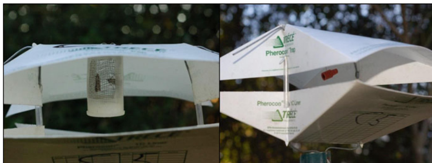
Fig. 14.3 Wing-type traps with sticky bottom panels initially baited with live females to survey for the invasive Cactus Moth, C. cactorum , until a pheromone-based lure was developed. Live females were changed every 3–5 days; the current lure is replaced every 4–6 weeks (Images courtesy of USDA-ARS-CMAVE, Tallahassee, FL)
