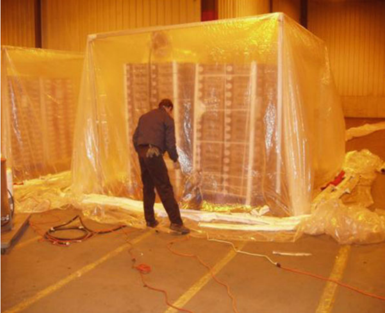
Fig. 10.5 Tarpaulin fumigation of break-bulk commodity
