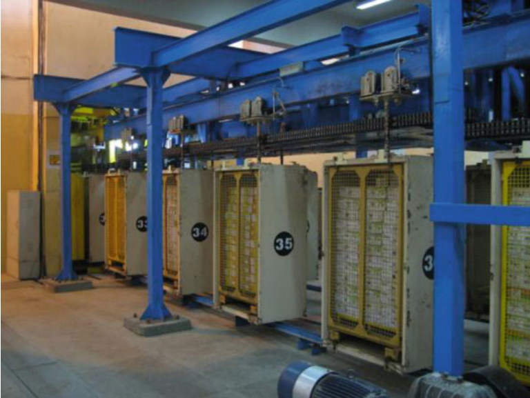
Fig. 10.17 Irradiation facility where “totes” filled with mangoes move along a conveyor to the protected cell ( left ), where the cobalt-60 source is located (Image courtesy CPHST, APHIS USDA.)
