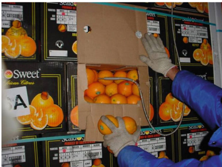
Fig. 10.8 Placement of pulp sensors before in-transit cold treatment of citrus (Image courtesy CPHST, APHIS, USDA)
