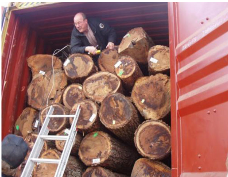
Fig. 10.6 Placement of monitoring leads and temperature sensors before a containerized tarpaulin fumigation of logs
