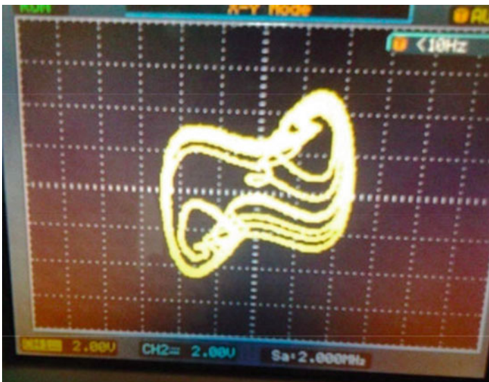
Fig. 2.9 The Asymmetric Logistic DDE \dot{x} = x_\tau(1 - |x_\tau|) realization. Parameters are: \tau = 3, x_0 = 0.9
