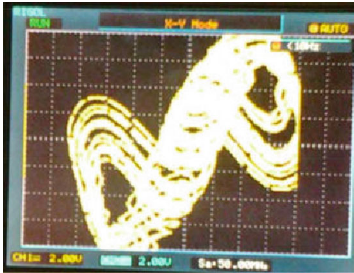
Fig. 2.6 The Ikeda DDE \dot{x} = \mu \sin(x_\tau - c) - x realization. Parameters are: \mu = 6 , \tau = 1 , c = 0 , x_0 = 0.1
