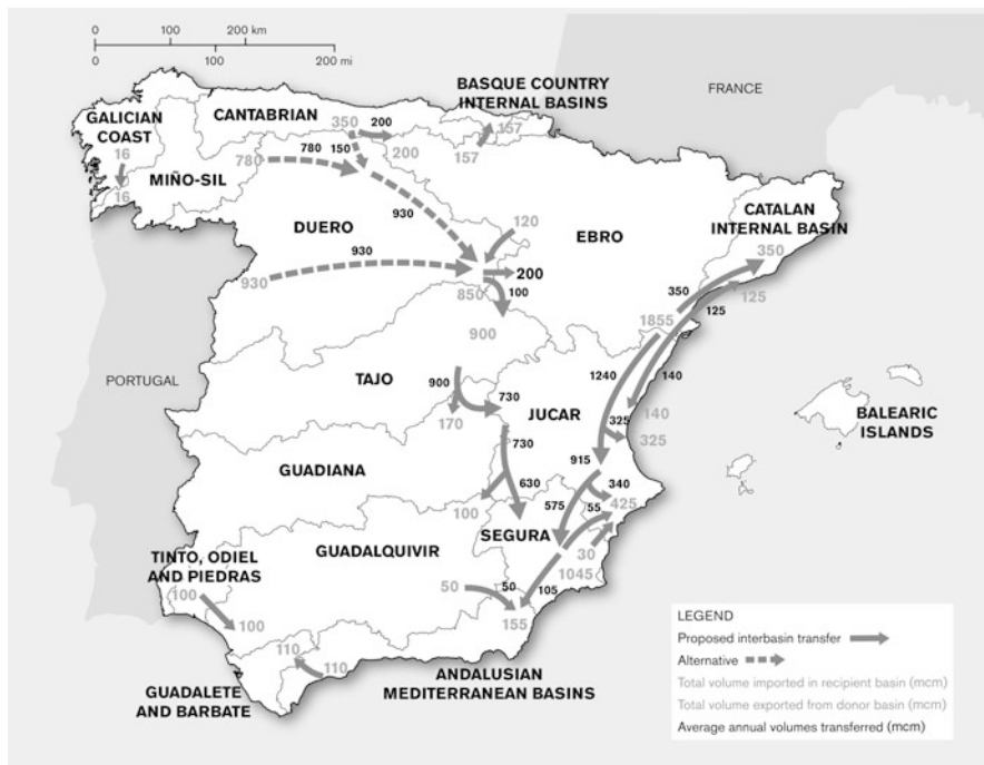
Fig. 13.2 National water grid as proposed in the 1993 draft National Hydrologic Plan (Source: MMA 2000)
