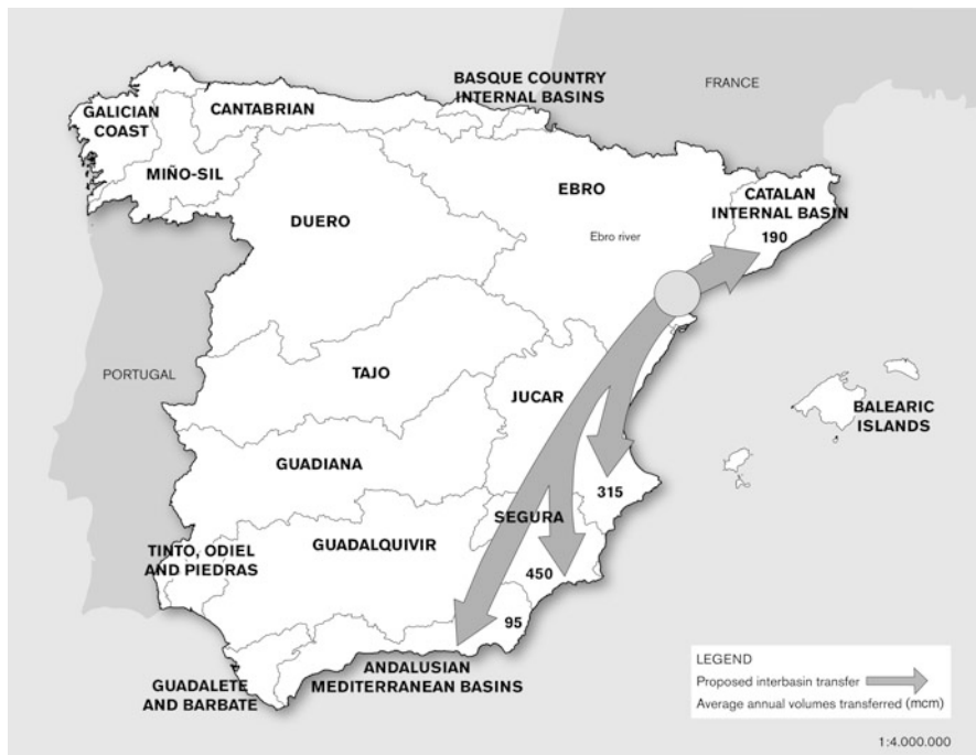
Fig. 13.4 The Ebro transfer proposed in the 2001 National Water Plan (Source: MMA 2001)
