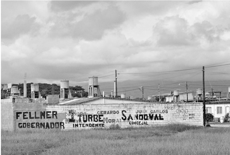
Fig. 15.1 Water tanks on the roof of buildings in Argentina, a sign of a lack of a water network. Names of candidates for elections are written on the walls (Source: Author)
