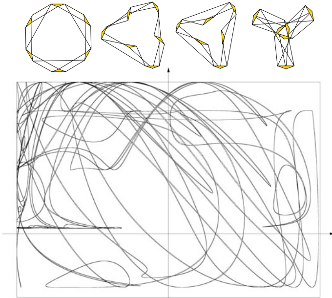
Fig. 3 Top The rigid wheel linkage on the left involves 10 loops. For the shown bar lengths, the tools of the CUIK suite determine that it can be assembled into 19 different configurations, including the four ones shown herein. Bottom The C-space of the wheel linkage with one bar removed, as computed by the mentioned tools. The C-space involves one isolated point and 15 one-dimensional components, which are here projected onto the sines of two link angles. A resultant polynomial describing such curve is expected to be of a very high degree
