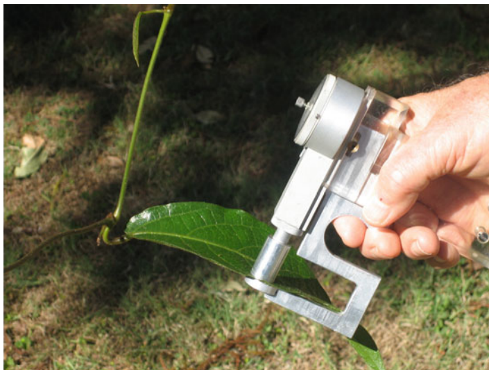
Fig. 6.2 The leaf penetrometer designed for use by school groups
