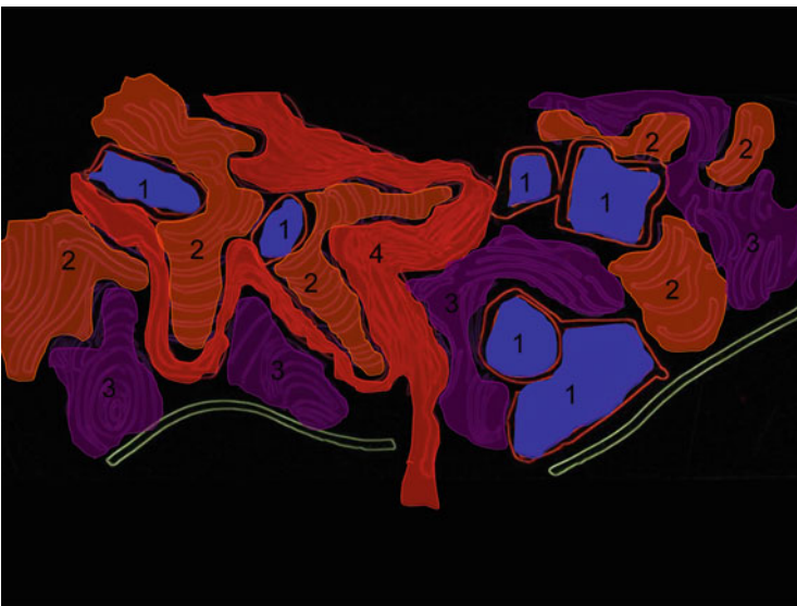
Fig. 10.6 Categorising slope types: flat (1), gentle (2), moderate (3) and steep (4) (Yu et al. 2006)
