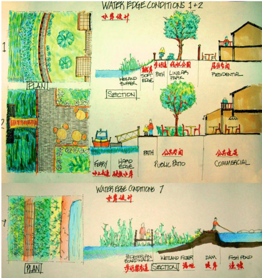
Fig. 9.24 Ecological soft edge and ferry landing edge and Boardwalk through wetland edge (Roggema and Van den Dobbelsteen 2006; Drawings: David Rousseau, Jinze Design Charrette 2006)
