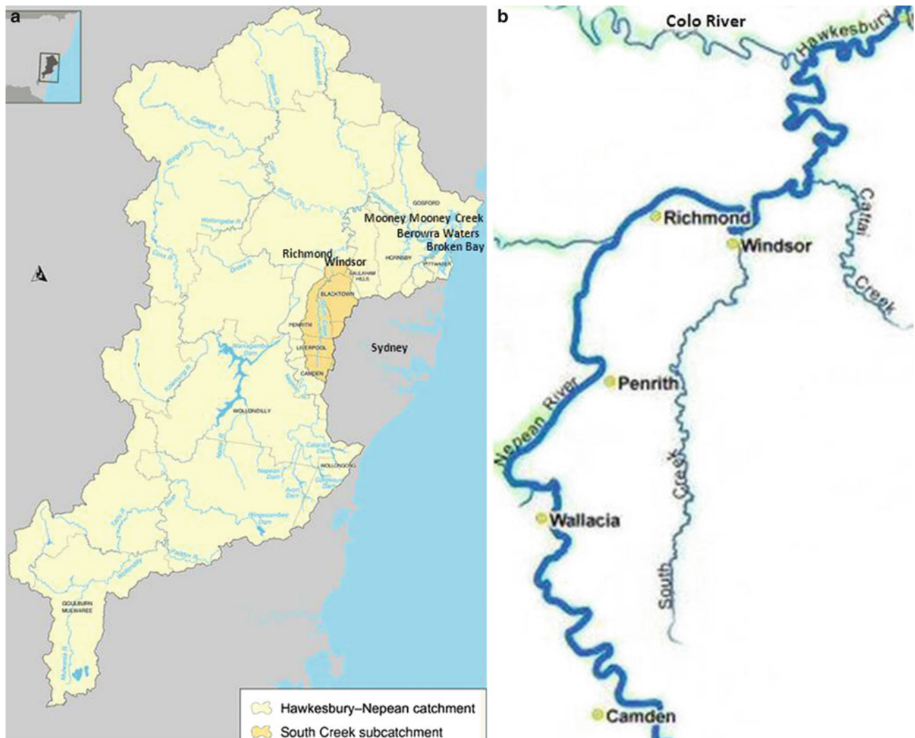
Fig. 1 (a) A location map of the Hawkesbury-Nepean River catchment. The tidal limit is located at about 140 km from the river mouth, near Windsor. (b) South Creek and Cattai Creek drain to the Hawkesbury Estuary the wastewater and wet weather runoff from Sydney western suburbs
