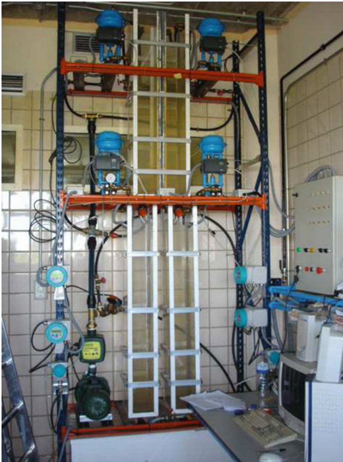
Fig. 25.4 The four tank process: the real plant diagram
